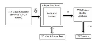
Figure 2. DVB-S2 test scenario (RF and subjective evaluation) [6].
