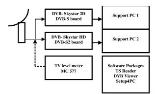
Figure 3. Configuration of the test system
