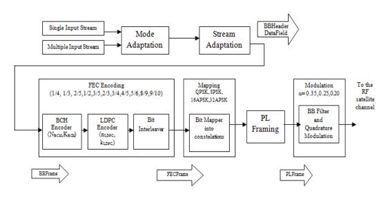
Figure 1. DVB-S2 transmission system. [3]
