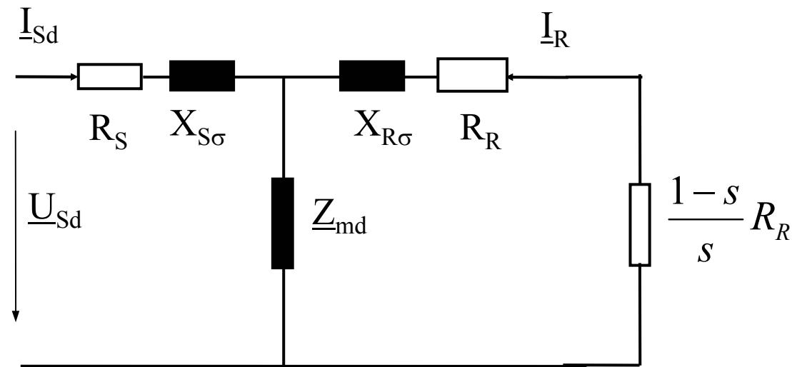
$$\underline{Z}_{ed} = \underline{Z}_S + \frac{\underline{Z}_{md} \cdot \underline{Z}_{Rd}}{\underline{Z}_{md} + \underline{Z}_{Rd}}$$
