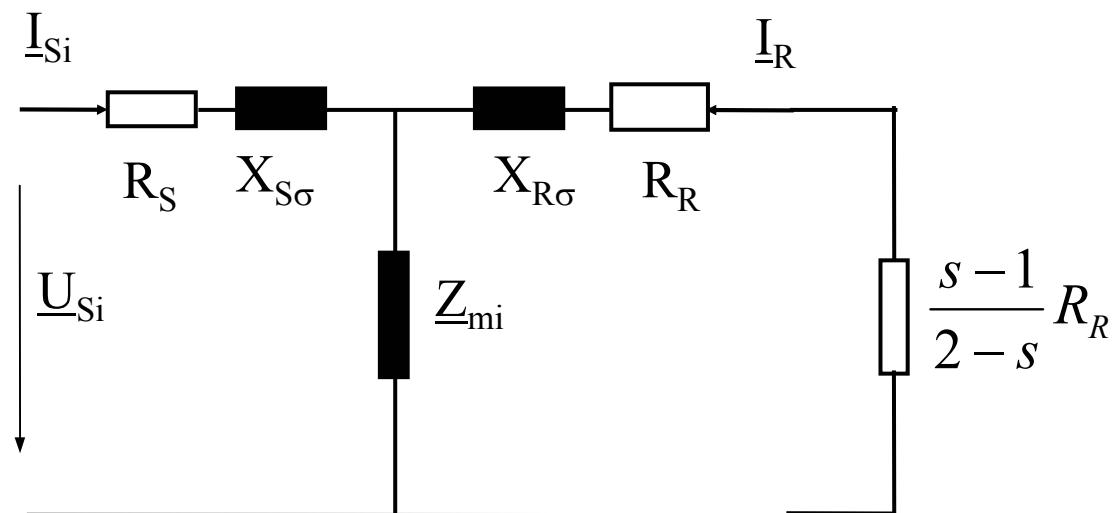
$$\underline{Z}_{ei} = \underline{Z}_S + \frac{\underline{Z}_{mi} \cdot \underline{Z}_{Ri}}{\underline{Z}_{mi} + \underline{Z}_{Ri}}$$
