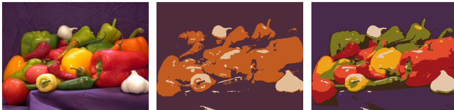
Figure 7.3 – Input color image and its segmentation using K=3 and K=10 centers
