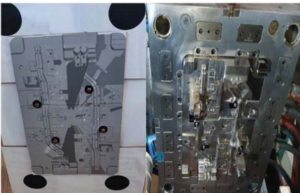
Figure 1. In the right-hand side an image of the original mold, and on the left-hand side the copy of the mold
