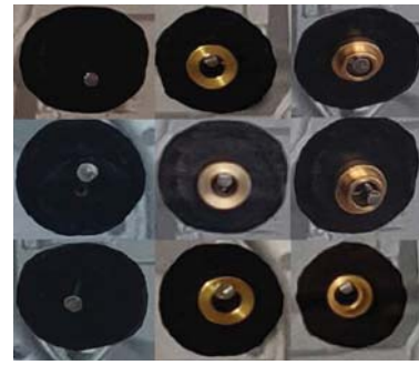
Figure 9. Multiple detection cases for the bushing ROI
