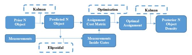
Fig. 2. Processing pipeline for obtaining the posterior N object density
