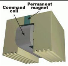
Figure 2. The mover module
