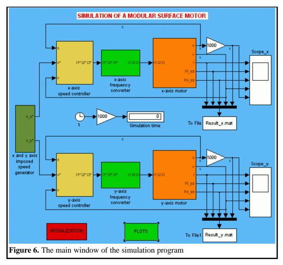
The simulated task was a typical pick and place type application. Such utilisation of the surface motors can be frequently seen in flexible manufacturing systems. The surface motors carry the product subassemblies from one overhead manufacturing device to another and precisely position the subassembly so that the overhead devices can perform their required actions.
