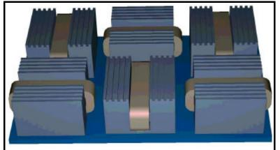
**Figure 3.** The arrangement of the modules in a three phase surface motor
