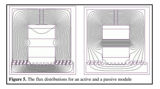
In figure 5 the magnetic flux distributions for an active, respectively a passive module and the platen part above are shown. It is easy to observe the manner, as the magnetic flux generated by the permanent magnet is directed through the air-gap in the first case and concentrated in the core branch under the magnet in the second case.
