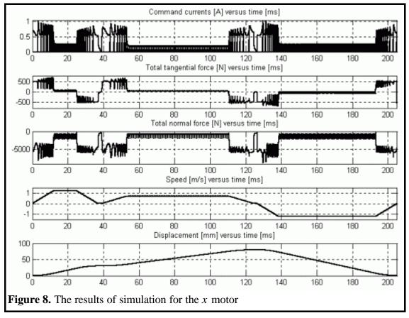
As it can be clearly seen in the figure, all the three imposed speed profiles were closely followed up. High tangential forces were needed for accelerating the mover. Due to the high force required the command currents for this stage have also significant values. After the mover was accelerated its imposed constant speed may be maintained by low tangential force.
