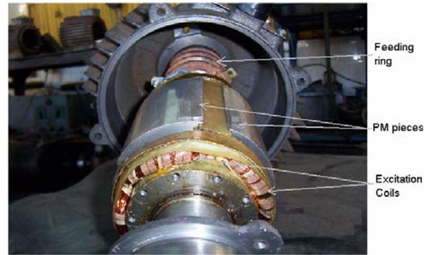
Fig. 8. HSM prototype rotor.
