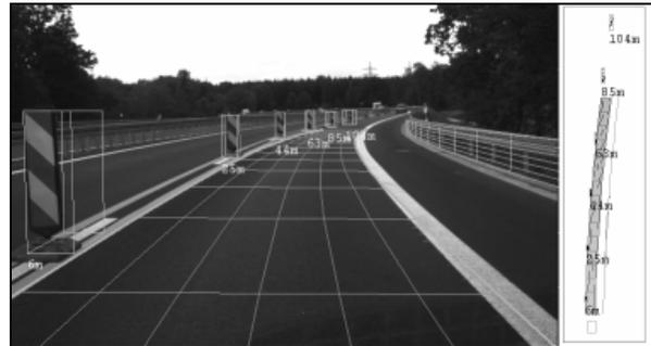
**Figure 10.** Highway scenario with lane and driving area delimiters (poles and fences) detected
