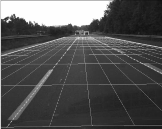
**Figure 6.** Current lane, side-lanes and very far obstacles detected on highways
