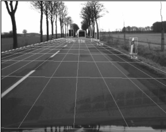
**Figure 7.** Current lane, opposite lane and far obstacles detected on partially marked country roads
