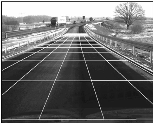
**Figure 8.** Results of lane detection on non-flat roads with vertical curvature
