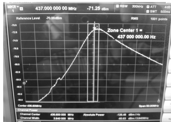
Figure 7. The noise signal generator through the three coaxial cells filter.
