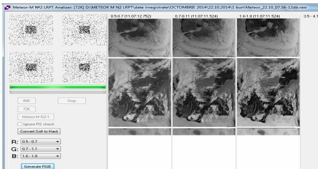
Figure 5. Unenhanced grayscale decoded images for the corresponding MSU-MR active channels.
