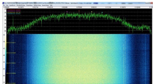
Figure 3. Sample of RF spectrum recorded using SDR-IQ receiver
