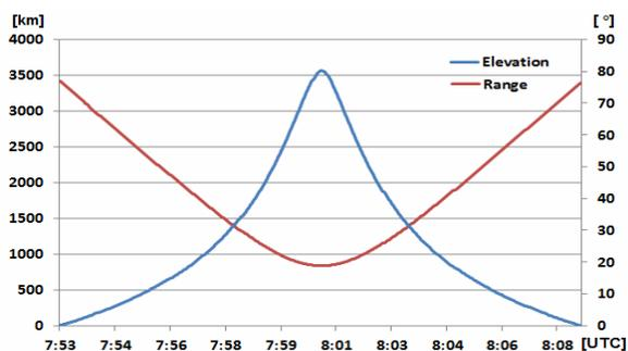
Figure 6. Range versus elevation for the corresponding Meteor-M N2 pass (10/22/2014, Orbit #1496)
