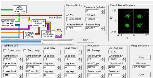
Figure 4. A well-defined four point constellation implies the successful QPSK demodulation of the received signal
