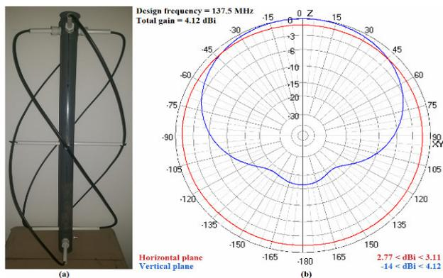
Figure 2. Fully assembled QFH antenna (a); Theoretical radiation diagram using 4NEC2 software (b)
