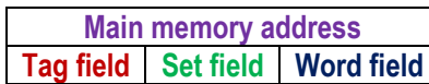
Figure 7. The format of an address from the main memory at set associative mapping
