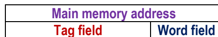
Figure 6. The format of an address from the main memory at fully associative mapping
