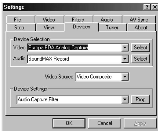
Fig.7. Selecting the BDA driver and video input
