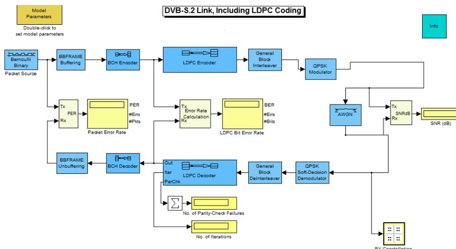
Figure 8. DVB-S2 model highlighting coding scheme [8]
