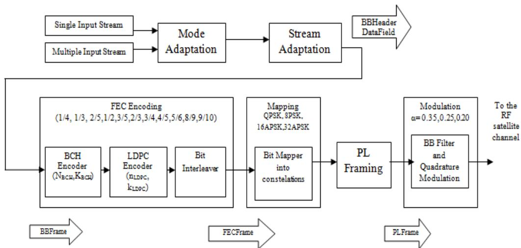
Figure 1. DVB-S2 transmission system. [3]
