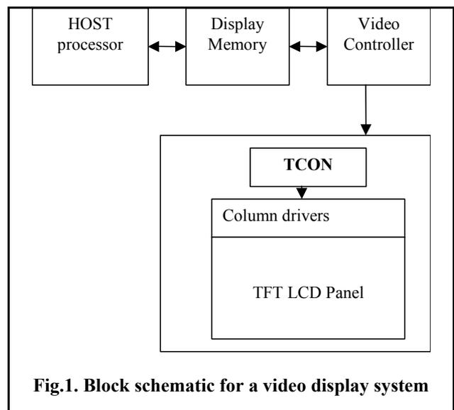
**Fig.1. Block schematic for a video display system**
