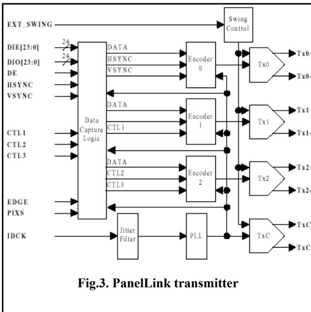
**Fig.3. Panellink transmitter**
