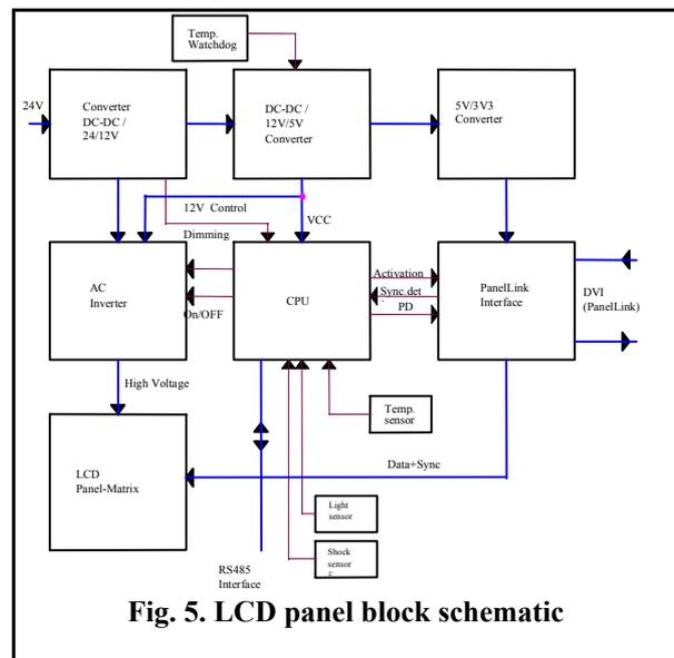
**Fig. 5. LCD panel block schematic**
