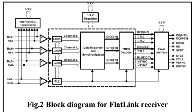
**Fig.2 Block diagram for FlatLink receiver**
