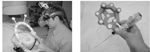
Figure 6. Two types of marker configurations. Left: A cantaloupe is placed into the head-clamp of a neurosurgical iMR operating room and viewed with the video-see-through HMD. Head tracking works in conjunction with nine retro-reflective markers that are reproducibly attached to the top of the head-clamp. Right: A biopsy needle which is equipped with a set of retro-reflective markers. The head-mounted tracker camera tracks this marker cluster to estimate the position and orientation of the needle. [13].
