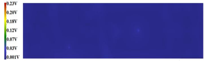
Figure 8. Visual representation of the propagation of the noise after using the capacitors from Table 1 for d=30mils(top) d=5mils (bottom).
