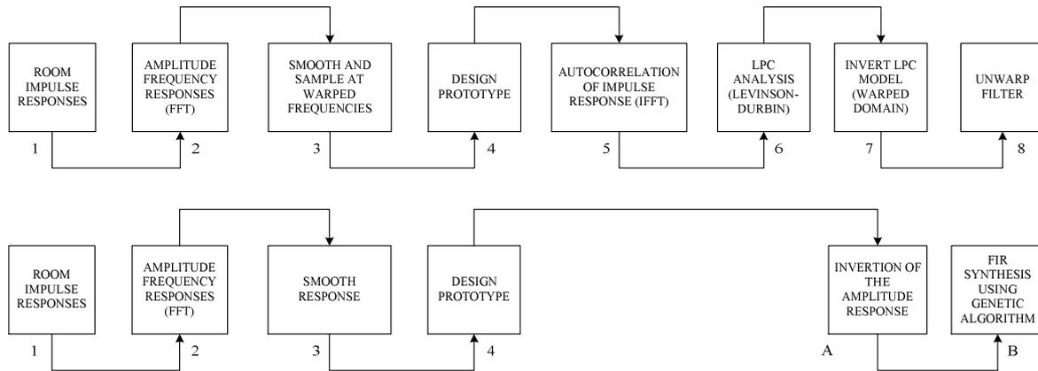
Figure 1. Multiple position room response equalization block diagram using the method from [8] (top) and the proposed method (bottom)
