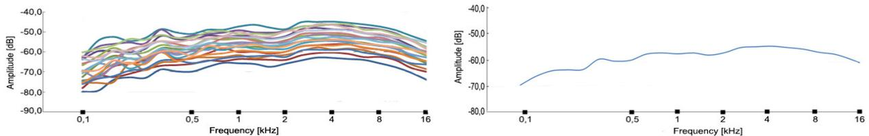
Figure 9. Measured magnitude responses with the equalizer inserted in the signal chain. a) the smoothed RTFs corresponding to the P1-P20 receiving points; b) the overall RTF for the audition area
