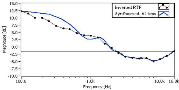
Figure 6. The desired magnitude response of the equalizer (dotted line) and the response of the synthesized FIR filter (continuous line)
