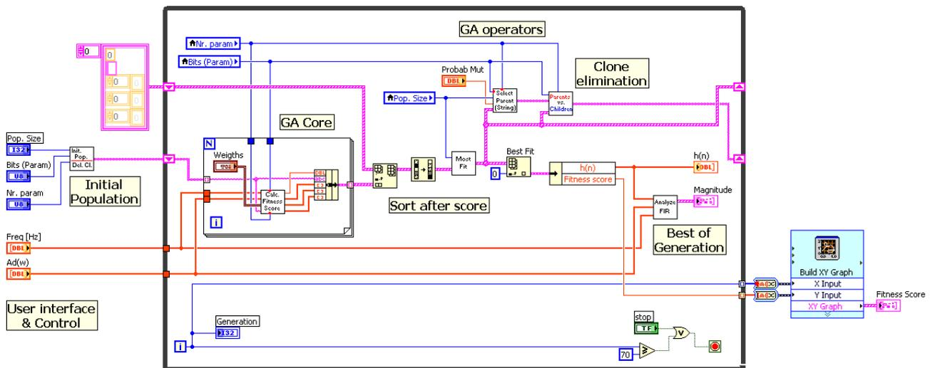
Figure 4. The LabVIEW diagram for implementing the proposed method for FIR filter synthesis
