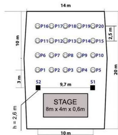
Figure 5. The floor plan of the recording studio
