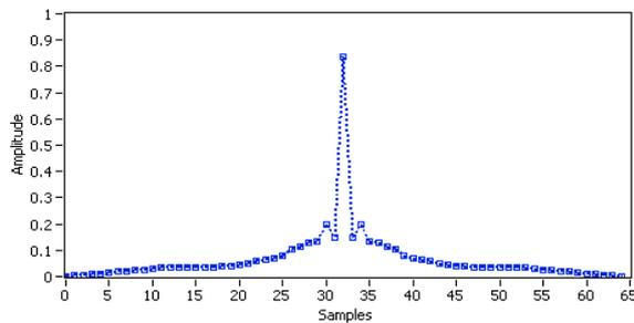
Figure 7. The impulse response of the synthesized 65-taps equalizer
