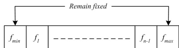
Figure 3. The structure of a chromosome that represents a filter: it comprises only the position in frequency of the samples used to synthesize the corresponding FIR filter
