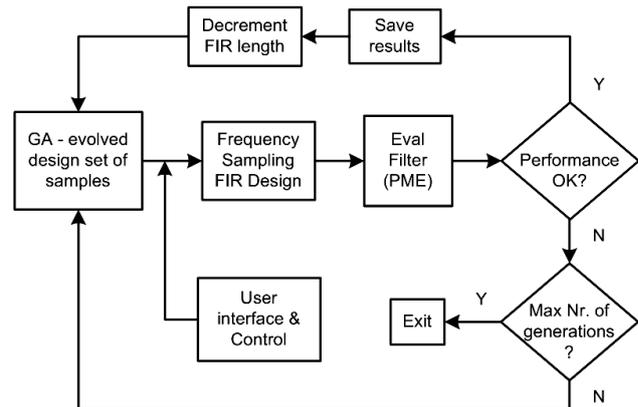
Figure 2. Block diagram of the proposed method for designing FIR filters with the magnitude responses that match the frequency characteristic defined by the user
