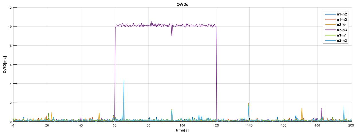
Figure 13. Additional OWD introduced on one of the links
