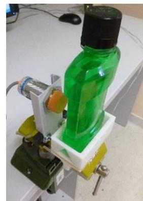
Figure 2. The new capacitive proximity sensor in combination with a specimen of ethylene-glycol
