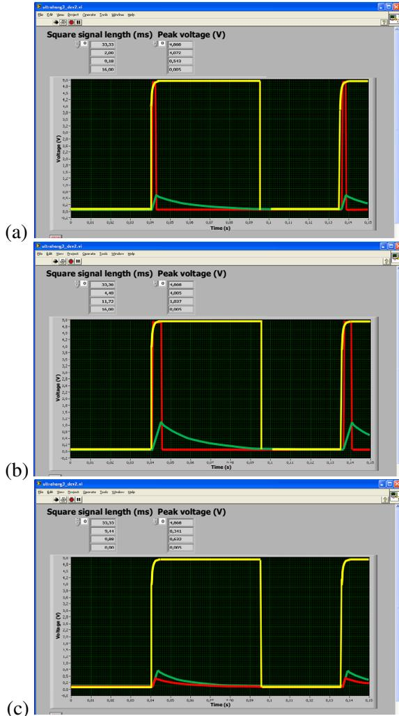
Figure 8. The front panel of the LabVIEW virtual instrument for data processing and visualization of the ultrasonic proximity sensing exercise. (a) Shorter echo time. (b) Longer echo time. (c) During the triangulating experiment: both receivers are in operation, and their integrated Echo pulses are measured
