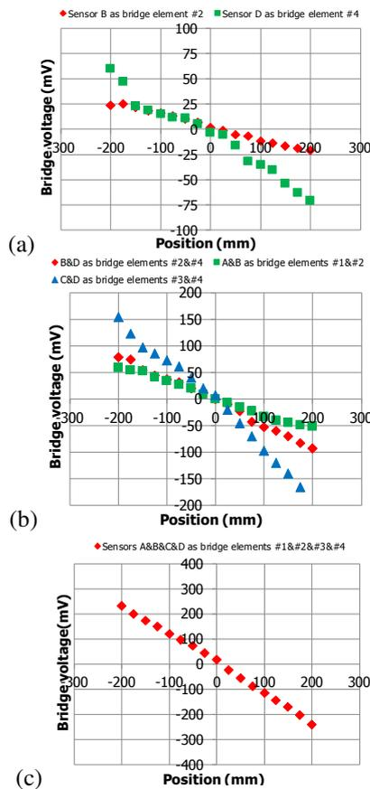
Figure 1. Characteristics of (a) the quarter, (b) the half and (c) the full Wheatstone bridge
