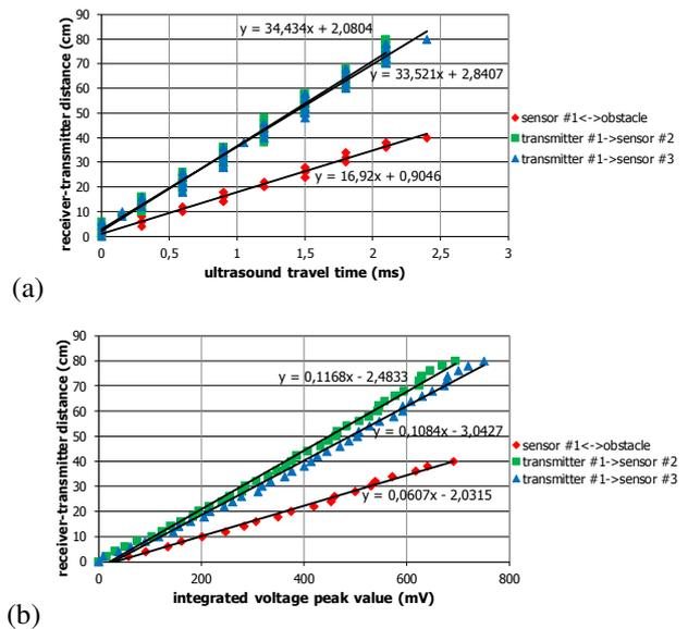
Figure 9. Plots of example data from the two-way and the one-way sensing setups: distance as the function of (a) echo pulse length (b) peak voltage of integrated waveform
