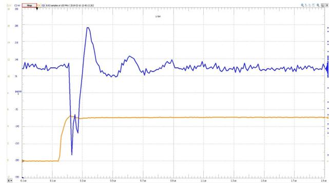
Figure 1. The rising slope of the Li-Ion battery
