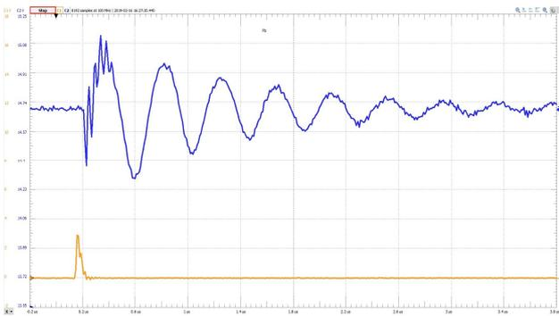
Figure 16. The needle pulse of the Lead-acid battery
