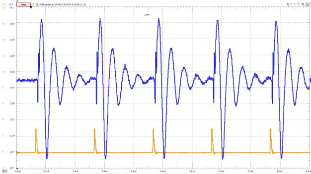
Figure 17. 500KHz pulses on the Li-Ion battery
