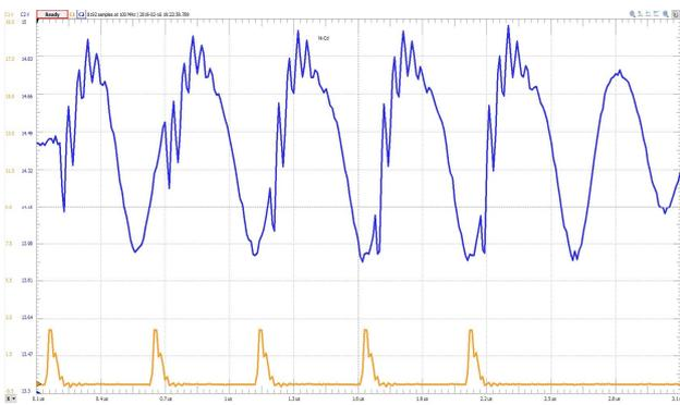
Figure 24. Pulse train of 2.05MHz on Lead-acid battery
