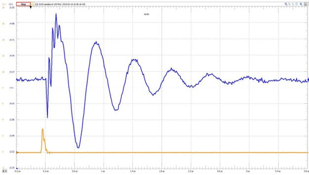
Figure 15. The needle pulse of the Ni-Mh battery
