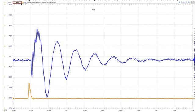
Figure 14. The needle pulse of the Ni-Cd battery
