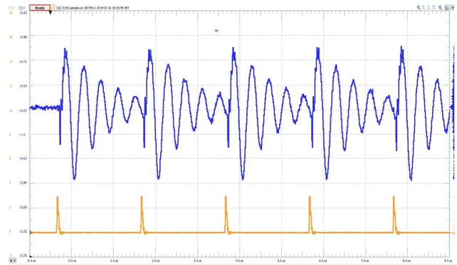
Figure 18. 500KHz pulses on the Ni-Cd battery
