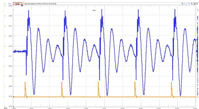
Figure 19. 500KHz pulses on the Ni-Mh battery
