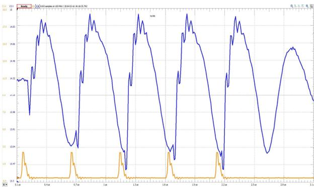
Figure 23. Pulse train of 2.05MHz on Ni-Mh battery
