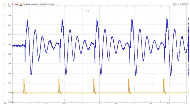
Figure 20. 500KHz pulses on the Lead-acid battery
