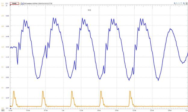
Figure 22. Pulse train of 2.05MHz on Ni-Cd battery
