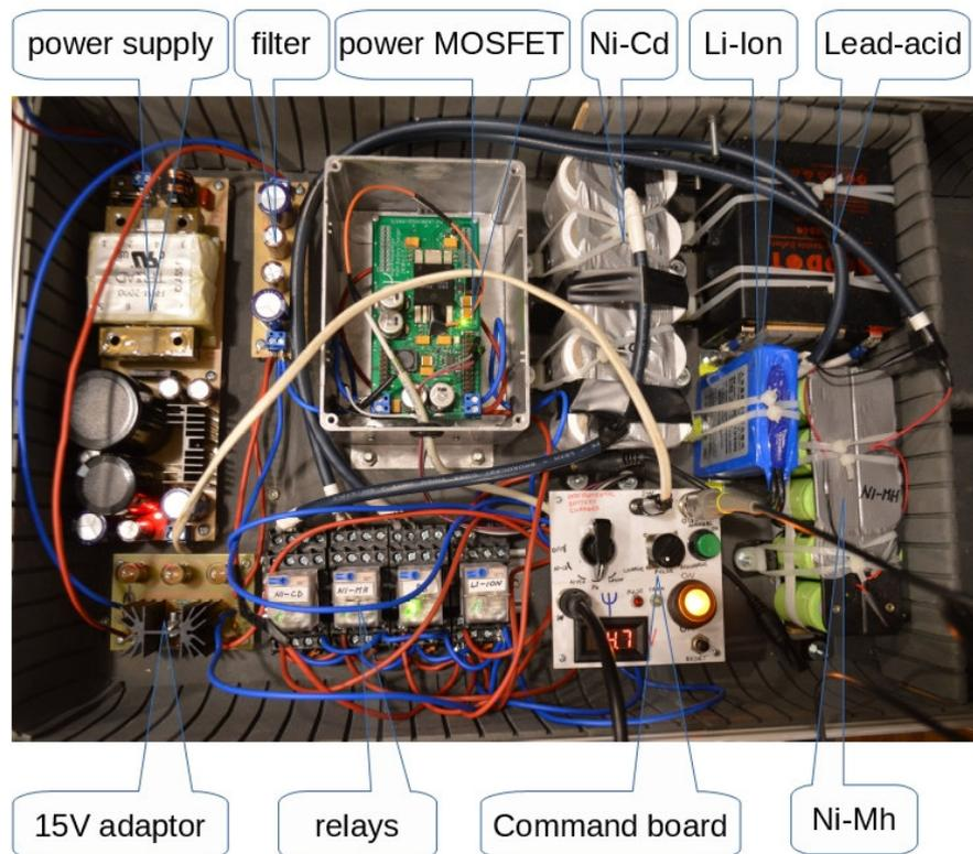
Figure 26. Hardware used in the experiments
