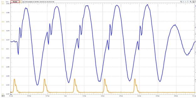
Figure 21. Pulse train of 2.05MHz on Li-Ion battery
