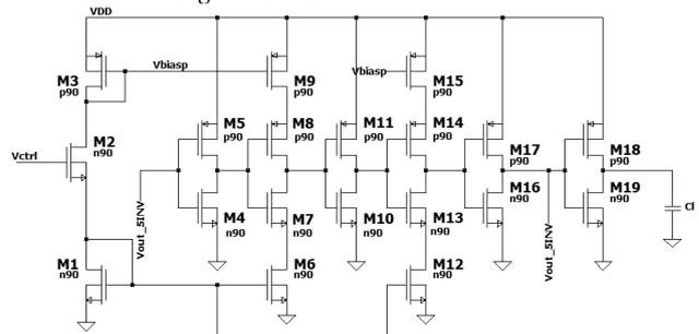
Figure 12. The combined VCO with inverter toward the load capacity
