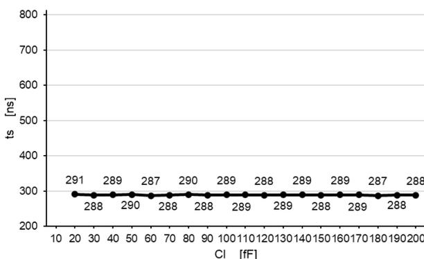
Figure 30. Variation of the phase-locked time according to the load capacity (Cl) for PLL with combined VCO, with an inverter to the output toward the load capacity
