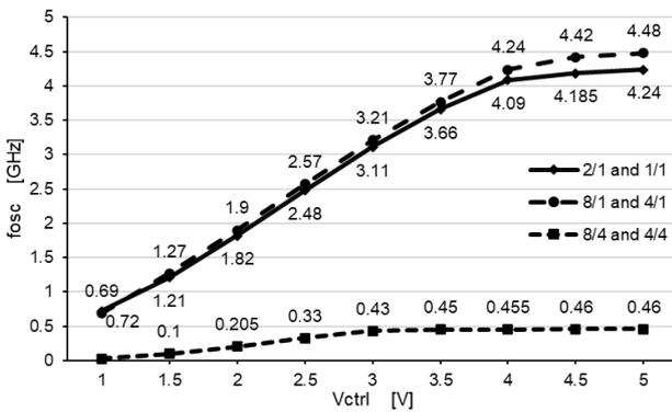
Figure 23. Variation of the oscillation frequency according to the control voltage ( $V_{ctrl}$ ) for simple VCO with an intermediate transistor in the current mirror, with an inverter to the output toward the load capacity
