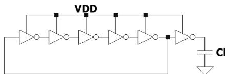
Figure 8. Ring oscillator with 5 inverters, a load capacity, and inverting gate at the output toward the load
