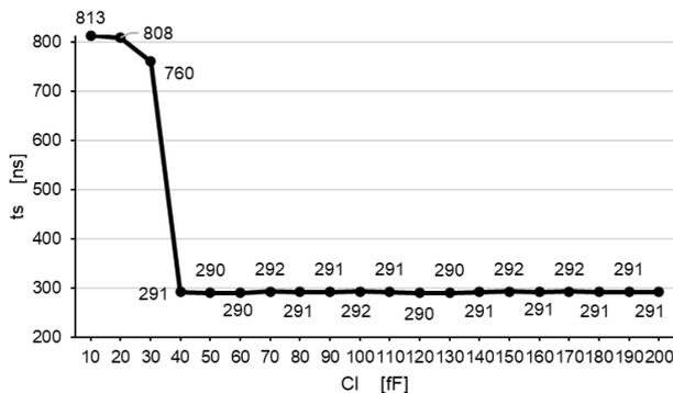
Figure 29. Variation of the phase-locked time according to the load capacity (Cl) for PLL with combined VCO
