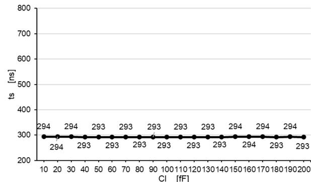
Figure 26. Variation of the phase-locked time according to the load capacity ( $Cl$ ) for PLL with simple VCO, with an inverter to the output toward the load capacity
