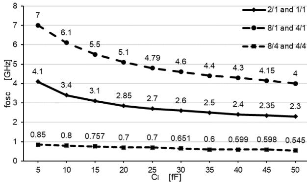
Figure 17. Variation of the oscillation frequency according to the load capacity ( $C_l$ ) for the ring oscillator with 5 inverters
