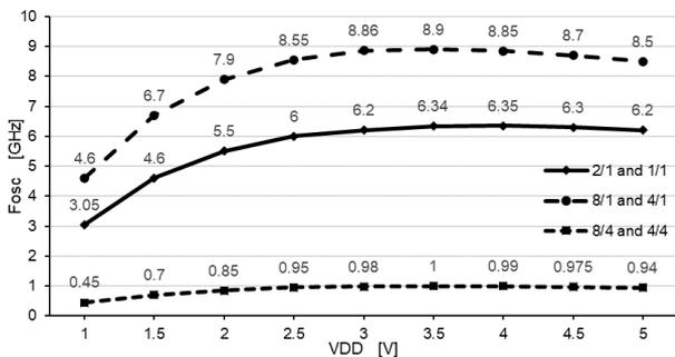
Figure 14. Variation of the oscillation frequency for the ring oscillator with 5 inverters depending on VDD
