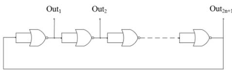
Figure 3. Ring oscillator implemented with NOR gates
