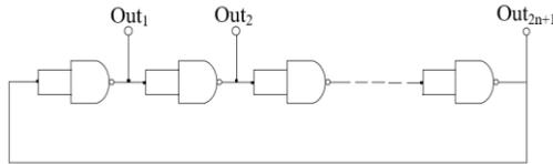
Figure 2. Ring oscillator implemented with NAND gates
