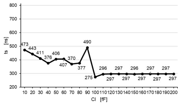
Figure 25. Variation of the phase-locked time according to the load capacity ( $Cl$ ) for PLL with simple VCO
