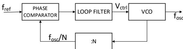
Figure 6. The Phase-Locked Loop
