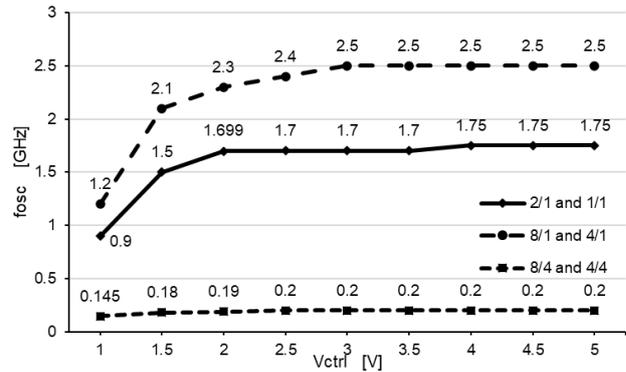
Figure 19. Variation of the oscillation frequency according to the control voltage ( $V_{ctrl}$ ) for simple VCO
