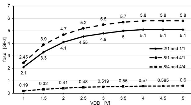
Figure 16. Variation of the oscillation frequency for the ring oscillator with 5 NOR gates depending on VDD
