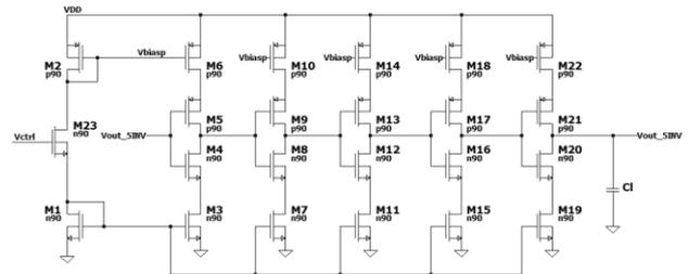
Figure 10. The VCO with 5 inverters and intermediate transistor
