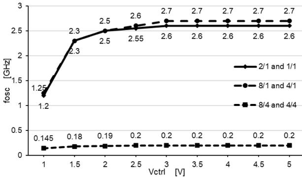
Figure 22. Variation of the oscillation frequency according to the control voltage ( $V_{ctrl}$ ) for simple VCO with an inverter to the output toward the load capacity
