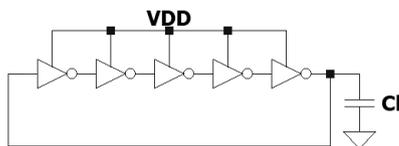
Figure 7. The ring oscillator with 5 inverters and a load capacity
