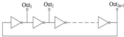
Figure 1. Ring oscillator implemented with inverters
