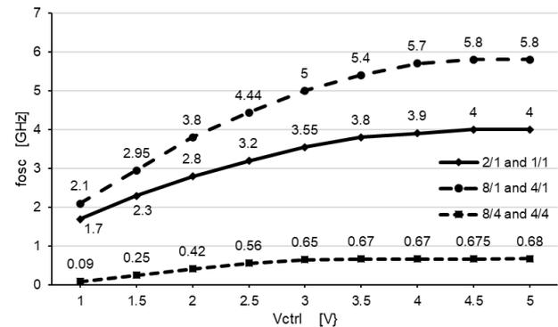
Figure 21. Variation of the oscillation frequency according to the control voltage ( $V_{ctrl}$ ) for combined VCO
