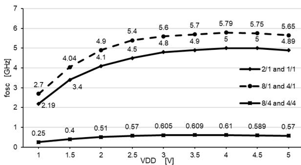
Figure 15. Variation of the oscillation frequency for the ring oscillator with 5 NAND gates depending on VDD
