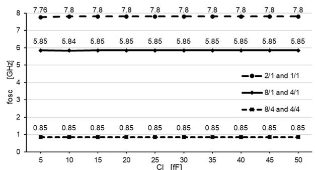
Figure 18. Variation of the oscillation frequency according to the load capacity ( $C_l$ ) for the ring oscillator with 5 inverters and reversing gate toward the load capacity
