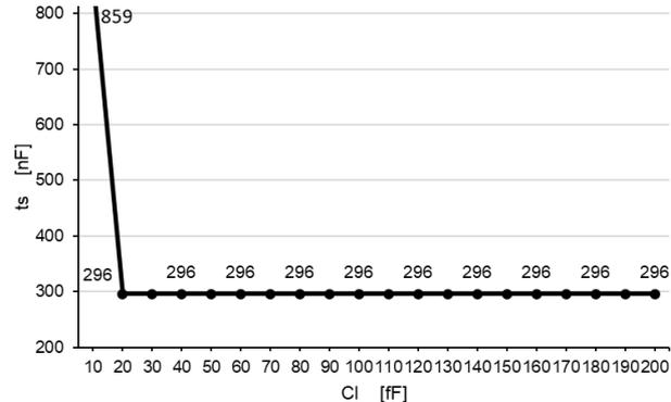
Figure 28. Variation of the phase-locked time according to the load capacity ( $Cl$ ) for PLL with VCO with an intermediate transistor in the current mirror, and with an inverter to the output toward the load capacity
