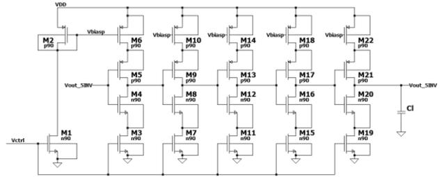
Figure 9. The VCO with 5 inverters
