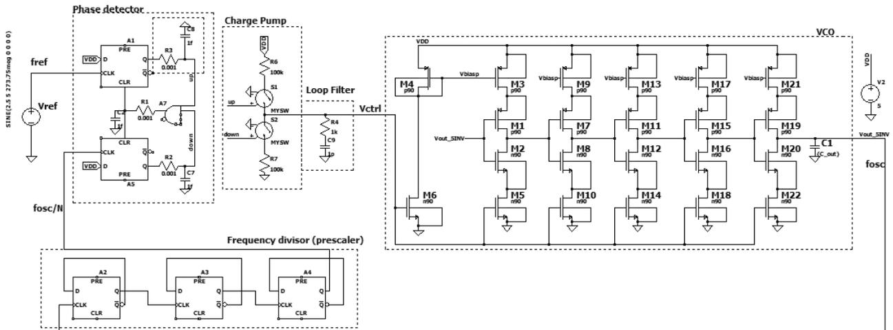
Figure 13. The Phase-Locked Loop
