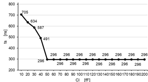
Figure 27. Variation of the phase-locked time according to the load capacity ( $Cl$ ) for PLL with VCO with an intermediate transistor in the current mirror
