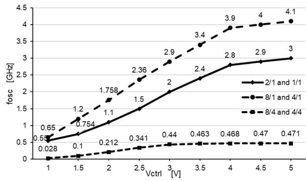
Figure 20. Variation of the oscillation frequency according to the control voltage ( $V_{ctrl}$ ) for VCO with an intermediate transistor in the current mirror
