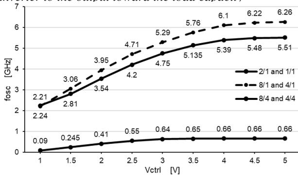
Figure 24. Variation of the oscillation frequency according to the control voltage ( $V_{ctrl}$ ) for combined VCO with an inverter to the output toward the load capacity
