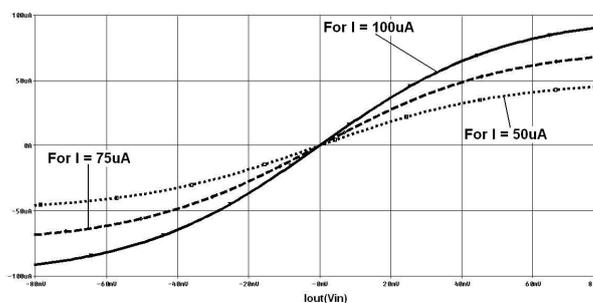
Figure 4. Hyperbolic Tangent cell DC\_sweep analysis
