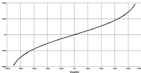
Figure 2. Hyperbolic Arctangent cell DC\_sweep analysis
