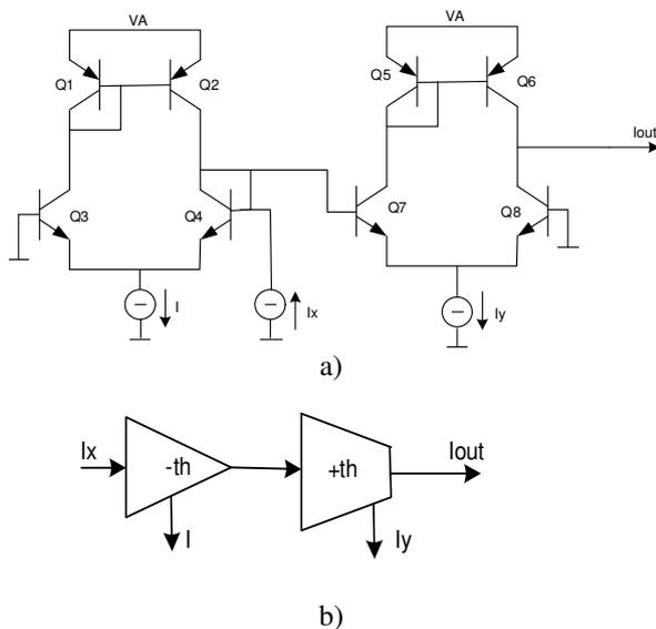
Figure 5. Two quadrant hyperbolic tangent domain analog current multiplier: a) schematic, b) block diagram
