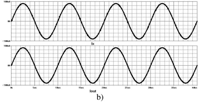
Figure 6. Analysis of the two quadrant current multiplier in the case of  $I_x=I$
