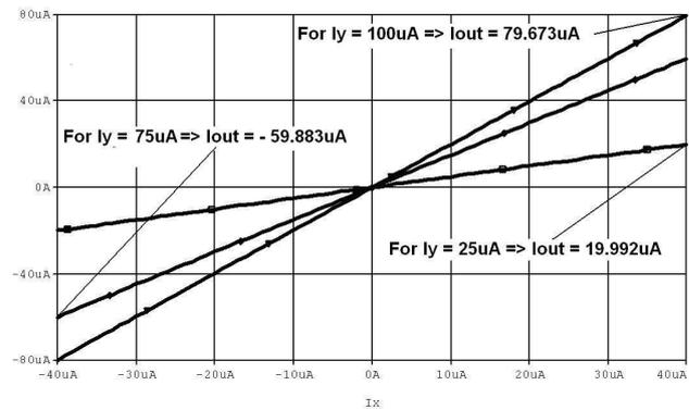
Figure 7. DC\_Sweep simulation for the two quadrant current multiplier in the  $I_x \neq I_y$  case
