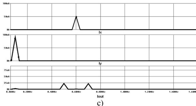
Figure 9. Analysis of the two quadrant current multiplier a) DC\_sweep b) Transient c) FFT
