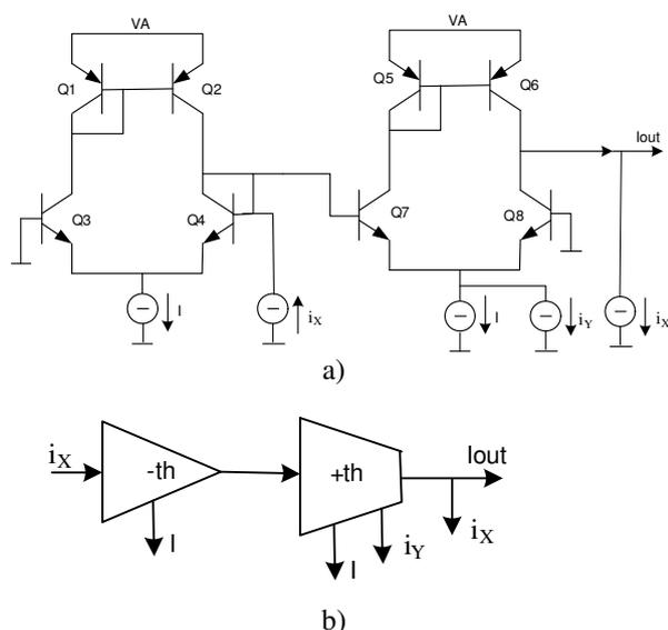
Figure 8. Four quadrant hyperbolic tangent domain analog current multiplier: a) schematic, b) block diagram
