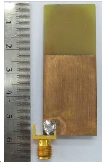
Fig-4: Back view of the fabricated antenna
