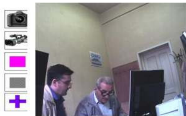
Figure 2. Application interface for visualization of images from camera and automatic record when motion is detected
