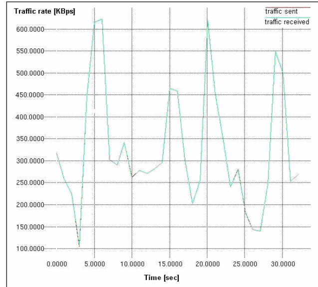
Figure 6. Test1-IPTV Traffic rate sent from the server and received at the client
