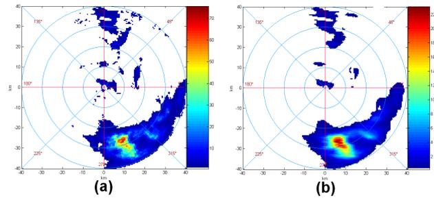
Figure 4. Rainfall [mm/h] (a) and rain attenuation [dB] (b).
