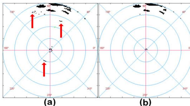
Figure 1. Clutter on a radar map (a) and clutter after the curing procedure (b).
