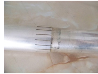
Figure 13. Coupling the fixed part of the coil to its mobile one
