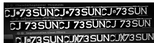
Figure 7. An example of segmentation output before cleaning filters applied, and afterwards
