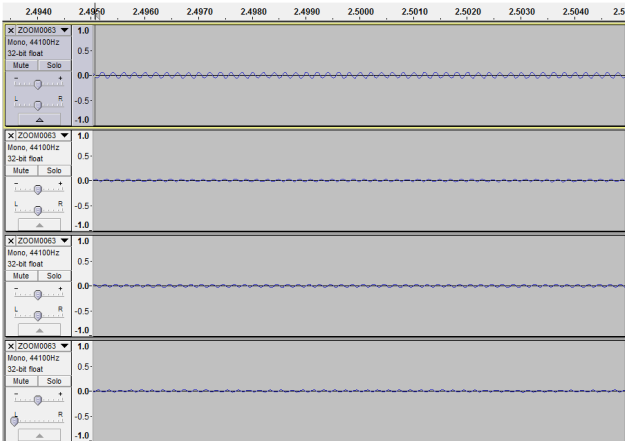
Figure 5. Acoustically designed room – sinusoidal signal with frequency 5 kHz (1st row - Mic 1 (N); 2nd row - Mic 2 (E); 3rd row - Mic 3 (S); 4th row - Mic 4 (V)).
