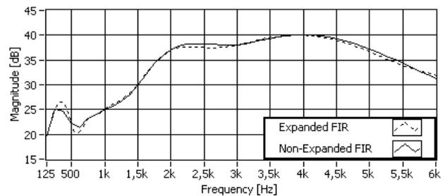
Figure 6. The audiogram approximation with Spline interpolation FIR filter
