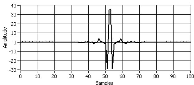
Figure 10. The impulse response of the Hermite interpolation FIR filter
