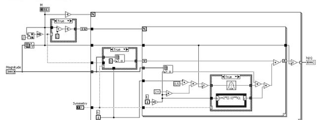
Figure 2. The block diagram of the coefficient vector computation ( $N$  even and FIR symmetric).
