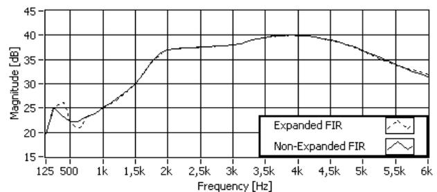
Figure 7. The audiogram approximation with Hermite interpolation FIR filter
