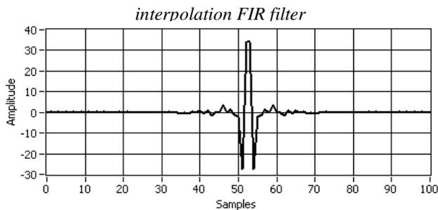
Figure 9. The impulse response of the linear interpolation FIR filter
