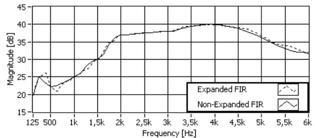
Figure 5. Audiogram approximation with cosine interpolation FIR filter
