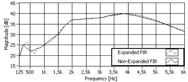
Figure 4. The audiogram approximation with linear interpolation FIR filter
