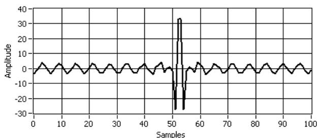
Figure 11. The impulse response of the rational interpolation FIR filter
