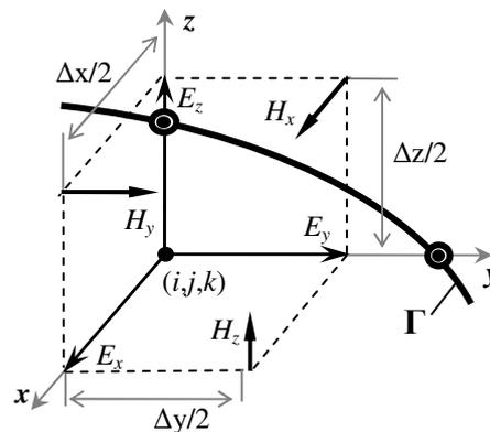
Figure 6. The radiated power was calculated on the curve  $\Gamma$  by using the interpolation.
