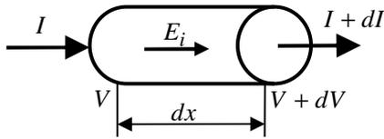
Figure 7. The equivalent circuit of a dipole's segment
