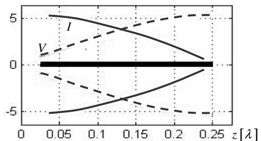
Figure 9. Current and potential distribution along the dipole.
