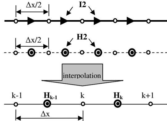
Figure 5. The currents through the dipole ( $I_2$ ), the magnetic field at double resolution ( $H_2$ ) and the magnetic field at Yee's resolution ( $H$ ).
