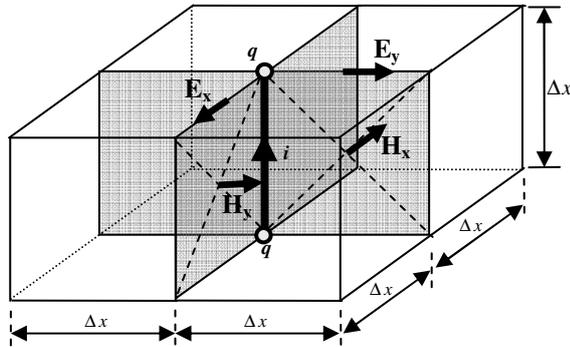
Figure 4. The connection of one segment of the dipole to the FDTD space.
