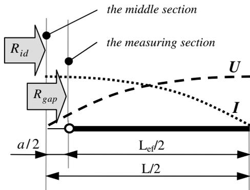
Figure 1. The correct measuring of the input reactance for a dipole with gap
