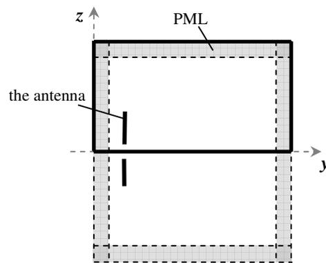
Figure 3. The dipole antenna in the infinite 3-D space (the outlined rectangle represents the modeled space).
