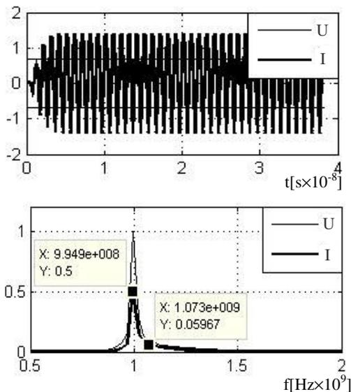
Figure 12. The voltage and the current at the input of the antenna, for  $\alpha_P = 0.99$
