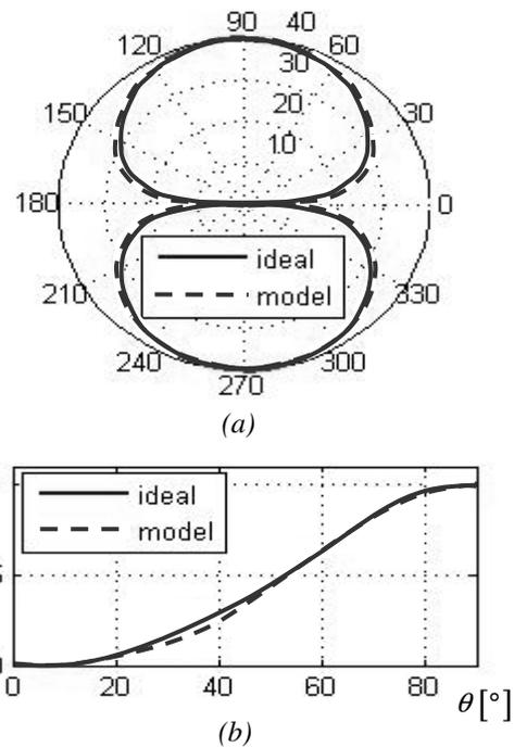
Figure 8. The radiation pattern: (a) polar representation (in dB); (b) linear representation.
