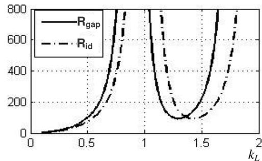
Figure 2. The input resistance of the dipole antenna without gap ( $R_{id}$ ) and the input resistance of a dipole with a gap of 10% ( $R_{gap}$ ) versus the length factor.
