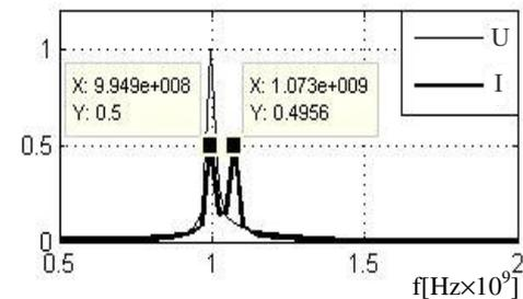
Figure 11. The voltage and the current at the input of the antenna, for  $\alpha_p = 1$
