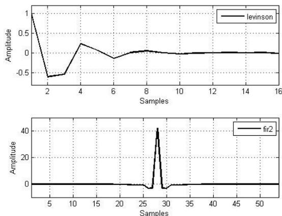
Figure 4. The impulse response in the case of levinson (16 coefficients) and fir2 respectively (54 coefficients).
