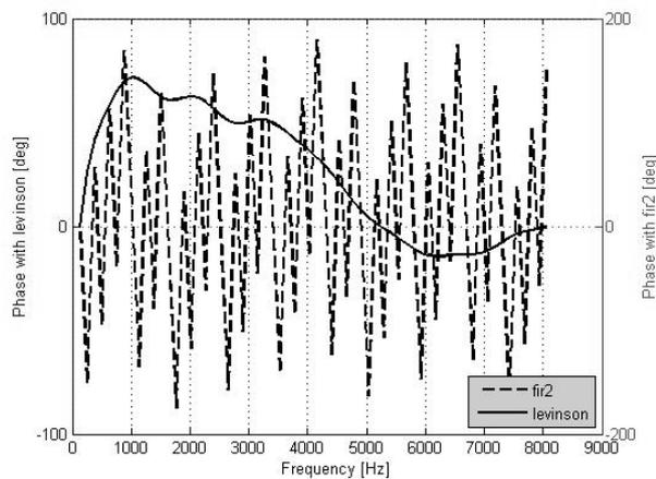
Figure 3. The phase characteristics of the filters synthesized with levinson (16 coefficients) and fir2 respectively (54 coefficients).
