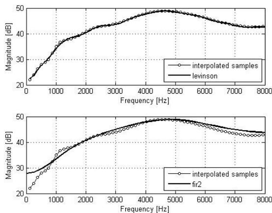
*Figure 1. The interpolated samples and the magnitude characteristics given by levinson and fir2 respectively (16 coefficients).*
