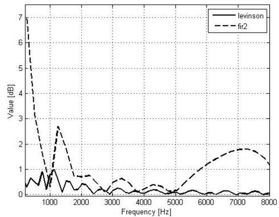
*Figure 2. The error in the approximation of the interpolated samples for levinson and fir2.m respectively (16 coefficients).*
