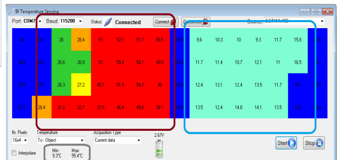
Figure 15: The data read from the 64 pixel MLX90620 sensor presented as a 16x4 pixel image.
