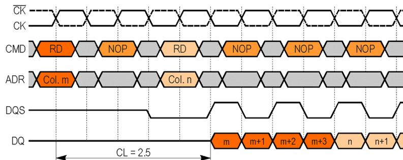
**Figure 4.25.** Consecutive burst *Read* operations for the DDR SDRAM memory.
