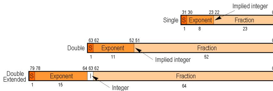
**Figure 3.28.** The single, double, and double extended formats defined by the IEEE 754 floating-point standard.
