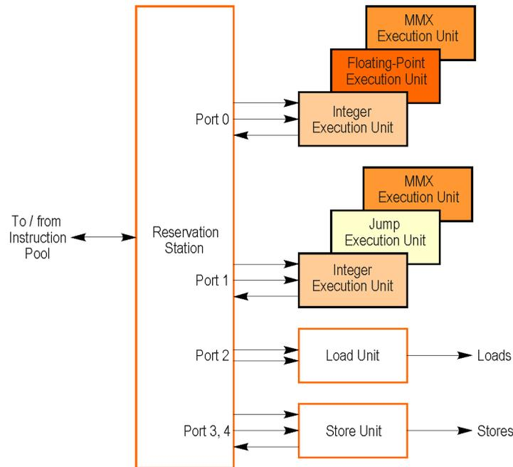
**Figure 5.18.** Intel Architecture processors dispatch/execute unit.
