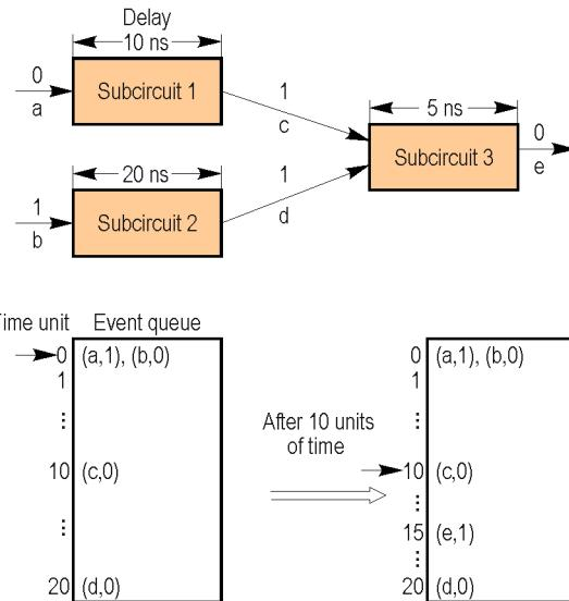
**Figure 2.11.** Simulation process.
