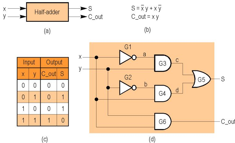
**Figure 2.4.** Different representations of a half adder: (a) block symbol; (b) Boolean equations; (c) truth table; (d) logic diagram.
