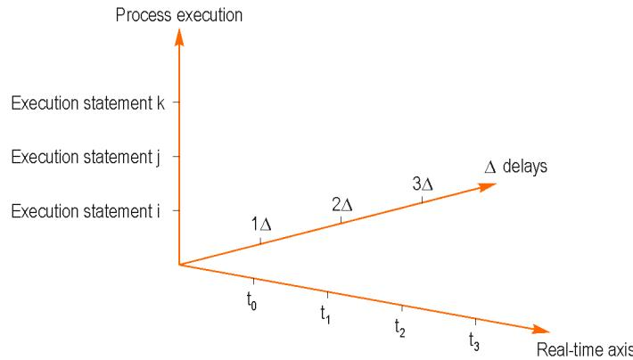
**Figure 2.8.** Three dimensions of time in VHDL.
