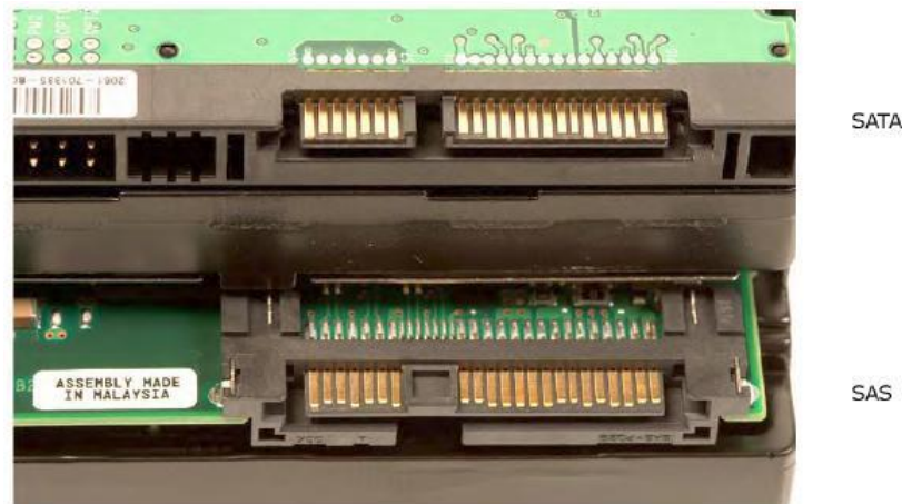
Figure 6.13. SATA and SAS disk drive connectors.
