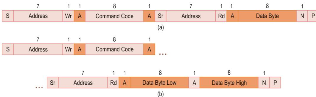
Figure 3.9. (a) *Read Byte* protocol; (b) *Read Word* protocol.
