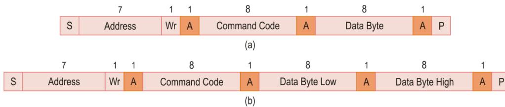
Figure 3.8. (a) *Write Byte* protocol; (b) *Write Word* protocol.
