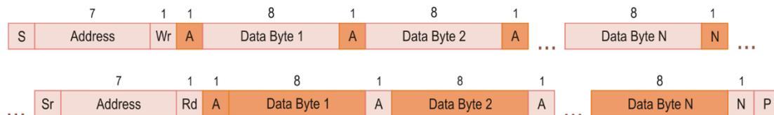
Figure 3.15. I<sup>2</sup>C combined format cycle.
