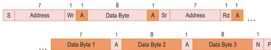
**Figure 3.22.** Write, read, start conversion cycle of the LTC2481 device.
