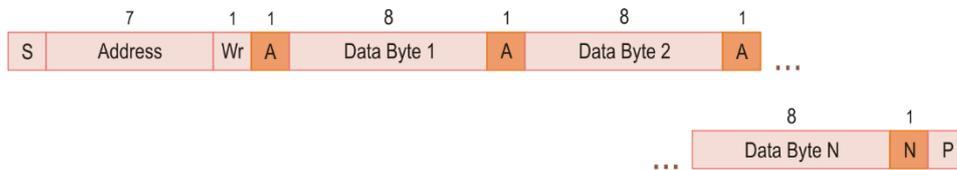
Figure 3.13. I<sup>2</sup>C write cycle.
