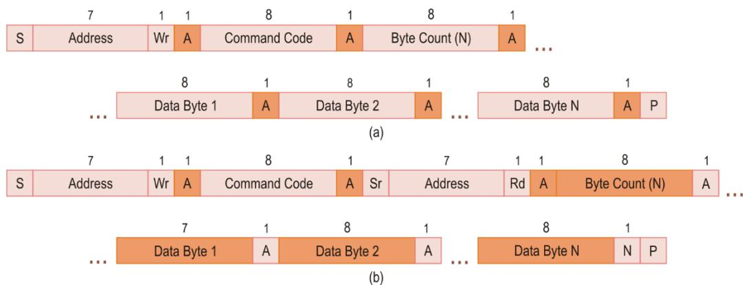
Figure 3.11. (a) *Block Write* protocol; (b) *Block Read* protocol.
