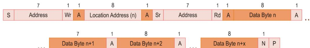
Figure 3.18. Sequential read cycle of the Microchip 24LC01B memory device.
