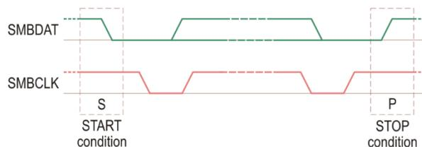
**Figure 3.3.** START and STOP conditions on the SMBus.
