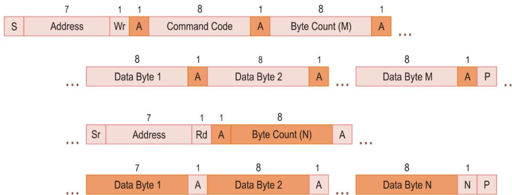
Figure 3.12. Block Write-Block Read Process Call protocol.
