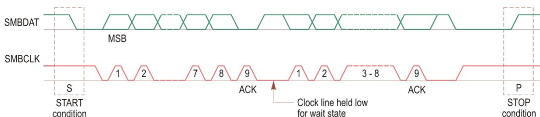
**Figure 3.4.** Example data transfer on the SMBus.
