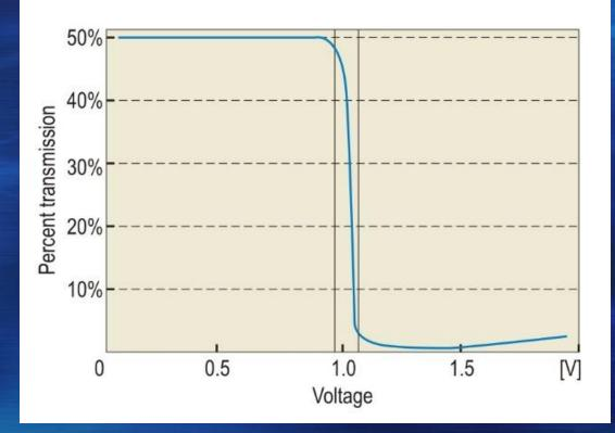
Percent transmission of light for an STN cell with a twist angle of 270°
