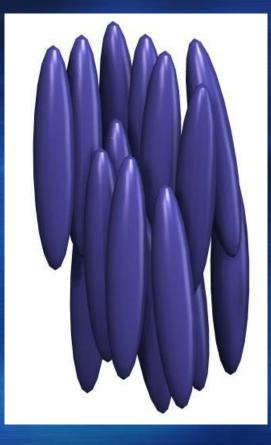
Nematic phase (N) Nema – thread; nemato – threadlike (Greek) Threadlike molecules No positional order Approximately parallel orientation order  $\rightarrow$ director Can be easily aligned by an electric field
