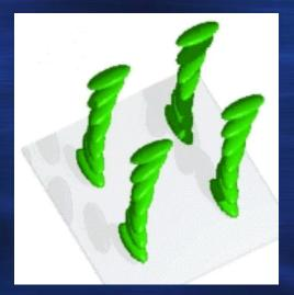
The polarized light passes through a TN liquid crystal layer
