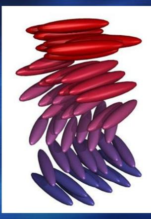
Cholesteric phase Typical for cholesterol esters  $\rightarrow$  cholesteric Chiral molecules: have no internal plane of symmetry Chiral nematic (N\*) Structure similar to a stack of 2D nematic layers The director in each layer is twisted
