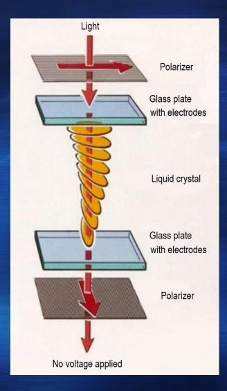
**Two polarizers** Two glass plates Two transparent electrodes TN liquid crystal layer No voltage is applied: The light is polarized by the first polarizer The polarizing direction is twisted with 90° The light will also pass through the second
