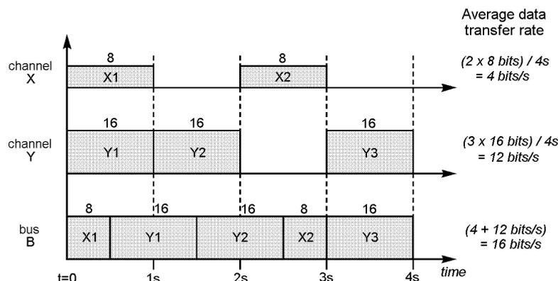
**Figure 2.** Merging channels  $X$  and  $Y$  into bus  $B$ .
