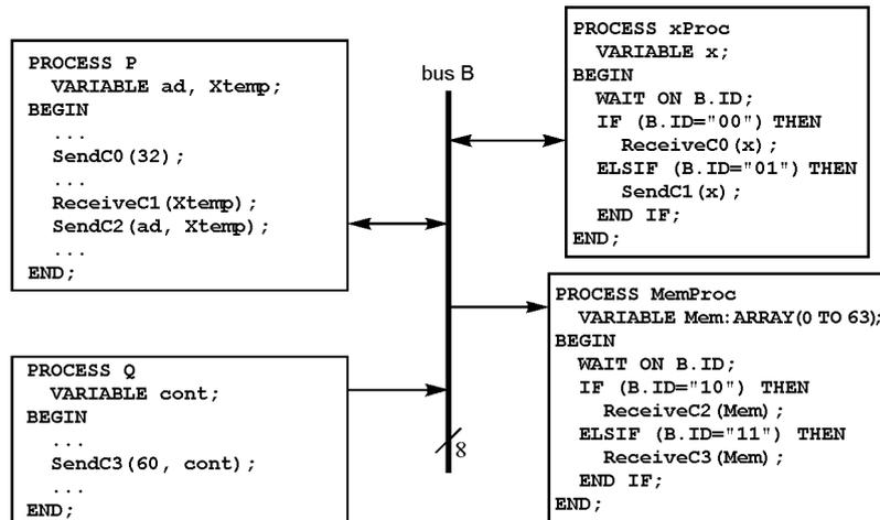
Figure 7. Refined specification after protocol generation.
