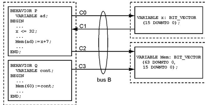
**Figure 5.** Processes accessing variables over channels grouped into a bus.
