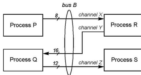
**Figure 1.** A typical bus formed by merging channels transferring data of different sizes between several processes.
