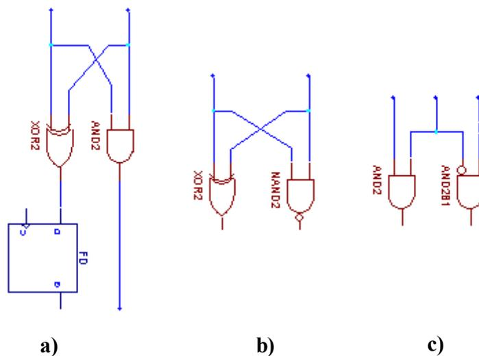
**Figure 3.** Three examples of Atmel logic cells with sub-configurations
