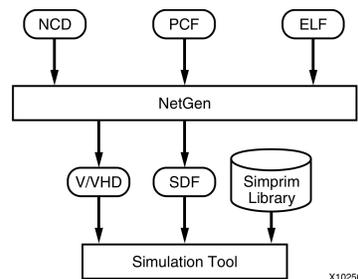
The FPGA Timing Simulation flow uses the following files as input:
