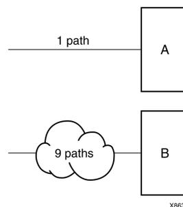
If an error is generated at the endpoints of A and B, the timing report would list one error for each of the end points.
