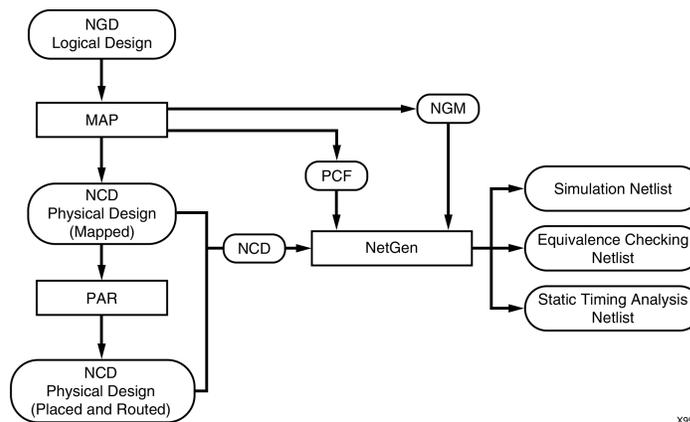
NetGen can be described as having three fundamental flows: simulation, equivalency checking, and third-party static timing analysis. This chapter contains flow-specific sections that detail the use and features of NetGen support flows and describe any sub-flows. For example, the simulation flow includes two flows types: functional simulation and timing simulation.
