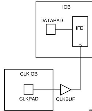
The pad CLKPAD of clock input component CLKIOB drives a global clock buffer CLKBUF, which in turn drives an input flip-flop IFD. The input flip-flop IFD clocks a data input driven from DATAPAD within the component IOB.
