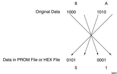
In a bitstream contained in a BIT file, the Least Significant Bit (LSB) is always on the left side of a byte. But when a PROM programmer or a microprocessor reads a data byte, it identifies the LSB on the right side of the byte. In order for the PROM programmer or microprocessor to read the bitstream correctly, the bits in each byte must first be swapped so they are read in the correct order.
