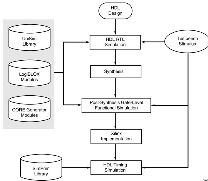
The three primary simulation points can be expanded to allow for two post-synthesis simulations. These points can be used if the synthesis tool cannot write VHDL or Verilog, or if the netlist is not in terms of UNISIM components. The following table lists all the simulation points available in the HDL design flow.
