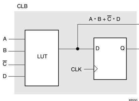
Observe that MAP has generated an active low (C) instead of an active high (C). Consequently, the Boolean output for the combinational logic is incorrect. When you run NetGen using the mapped.ngm file, you cannot detect the logical error because the delays are back-annotated to the correct logical design, and not to the physical design.
