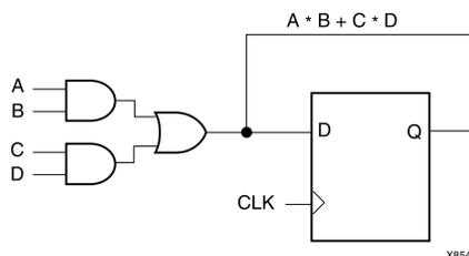
Observe the Boolean output from the combinational logic. Suppose that after running MAP for the preceding circuit, you obtain the following result.
