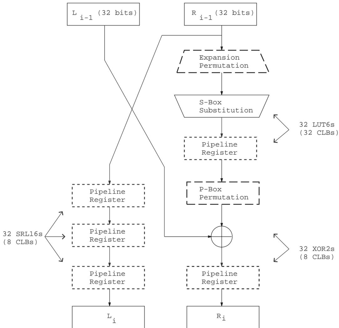
Figure 5: A Pipelined JBits DES Round
