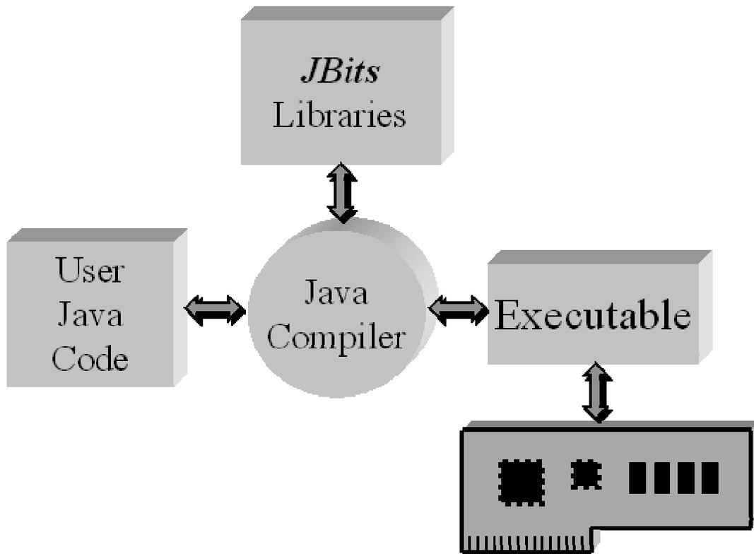
**Figure 1:** The *JBits* design flow.
