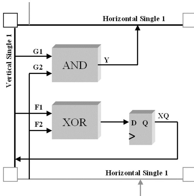
**Figure 4:** The counter cell circuit.
