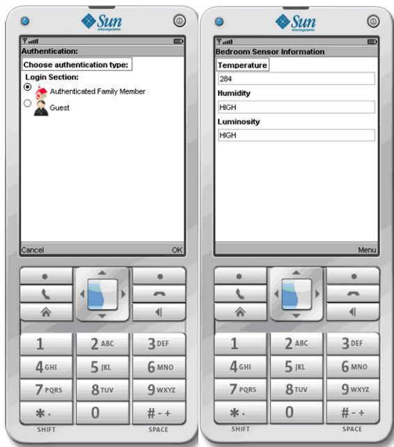
Figure 8. Mobile Agents Interface on Sun Java Wireless Toolkit (login – left, sensor information monitoring - right)
