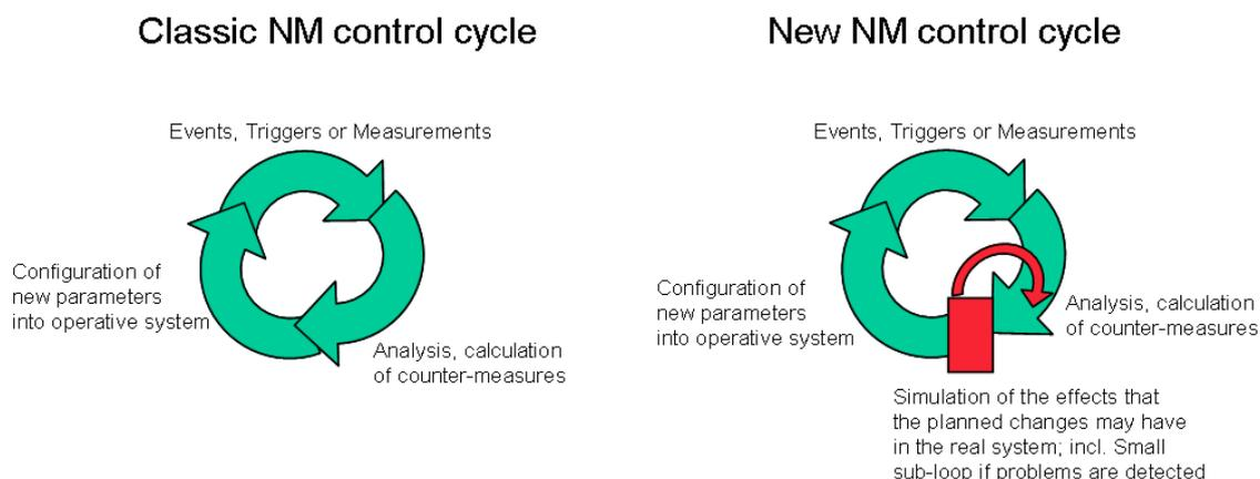
Figure 5-13: Classical and enhanced INM control cycle
