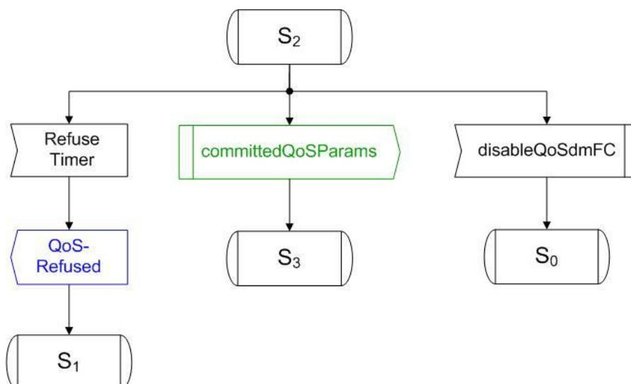
Figure A-5: QoSdmFC, state S2: top-down cross-layer
