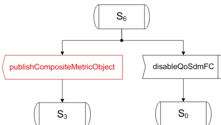
Figure A-9: QoSdmFC, state S6: composite metric published as a service
