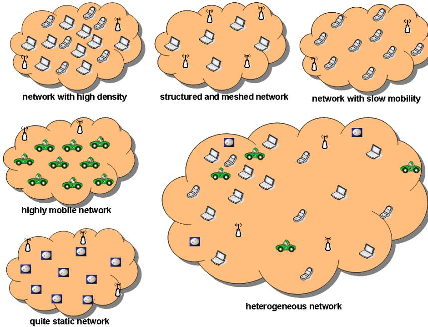
**Figure 5-9: Different types of wireless multi-hop networks**
