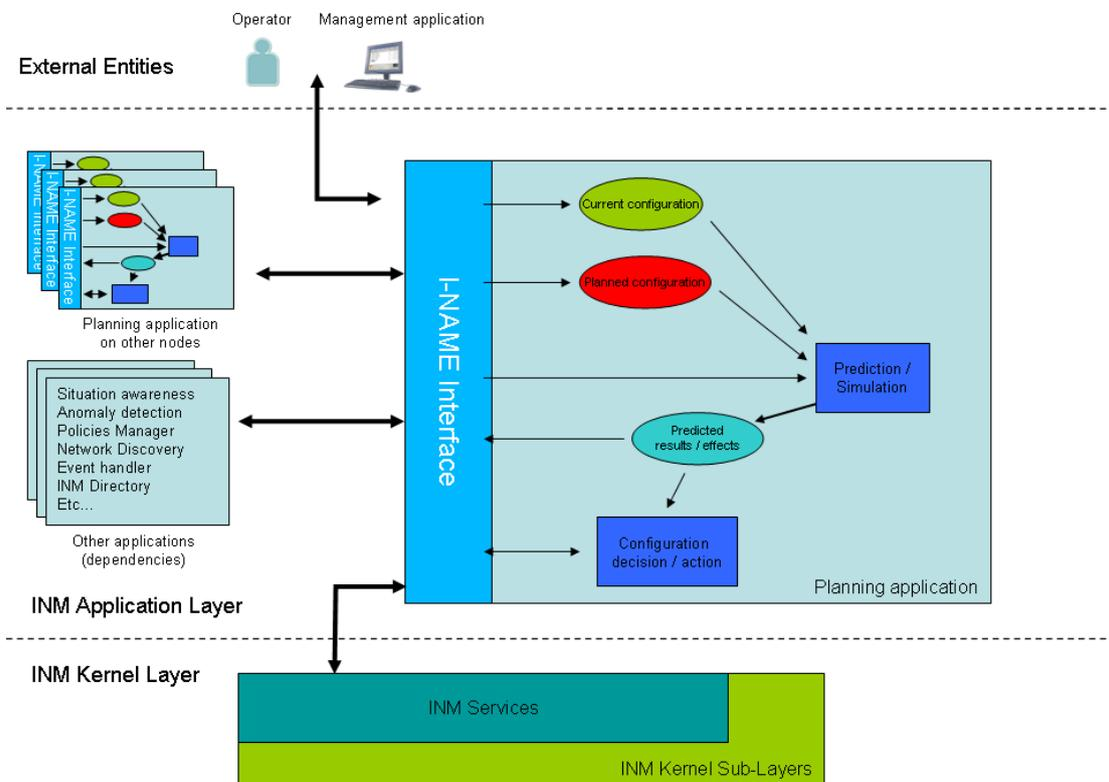
Figure 5-12: Architecture and external interfaces of the Network Configuration Planning application
