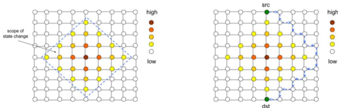
**Figure 5-21: Congestion notification based on frequency change**
