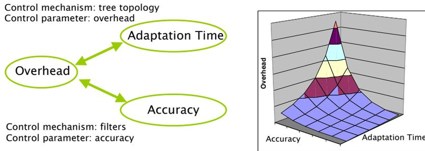
**Figure 4-9: Performance trade-offs in decentralized monitoring. The figure on the right shows the border of the feasible region for a protocol such as A-GAP**
