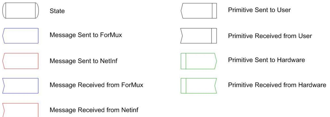
Figure A-2: QoSdmFC: messages and primitives using SDL
