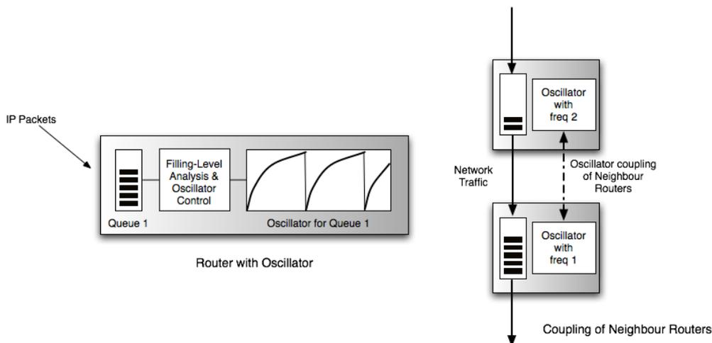
**Figure 5-20: Approach and coupling of routers (simplified view)**
