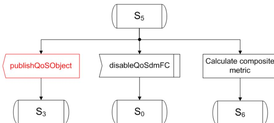
Figure A-8: QoSdmFC, state S5: QoS parameters published as a service
