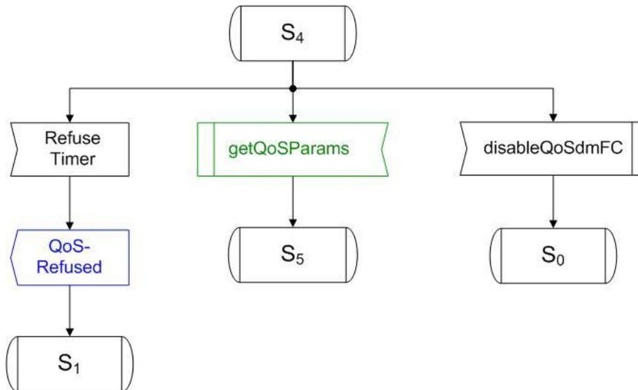
Figure A-7: QoSdmFC, state S4: bottom-up cross-layer
