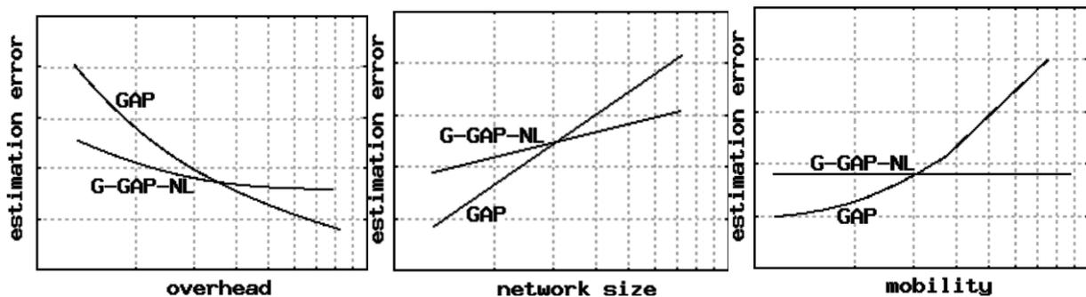
Figure 4-4: Comparison of tree-based (GAP) and gossip-based (G-GAP-NL) protocols for real-time monitoring: qualitative results from simulation study
