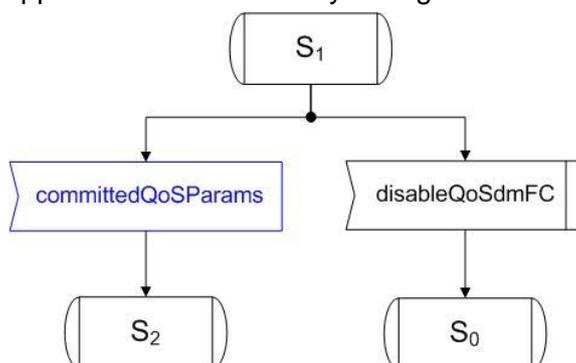
Figure A-4: QoSdmFC, state S1: waiting for top-down cross-layer request
