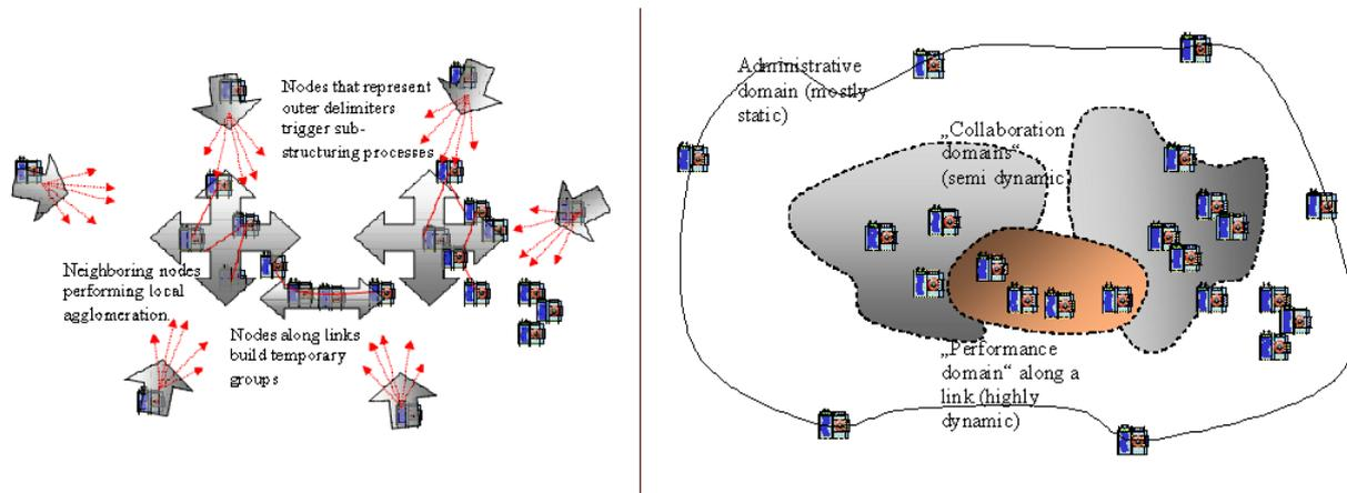
**Figure 3-13: Emergence of structure by using outside-in and inside-out self-structuring processes of an INM-enabled network (left: preparation signalling; right: established domains)**
