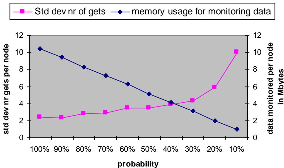
Figure 5-17: Standard deviation and amount of monitoring data gathered.
