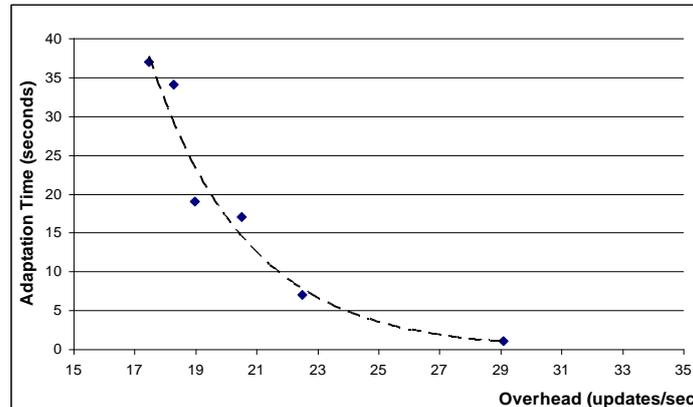
**Figure 4-10: Adaptation time as a function of the incurred overhead for a network of 200 nodes**
