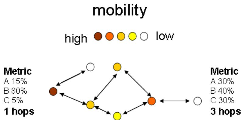
**Figure 5-11: Example for metric weighting according against mobility**
