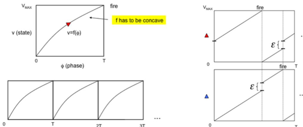
Figure 5-19: Oscillator model of Mirello & Strogatz
