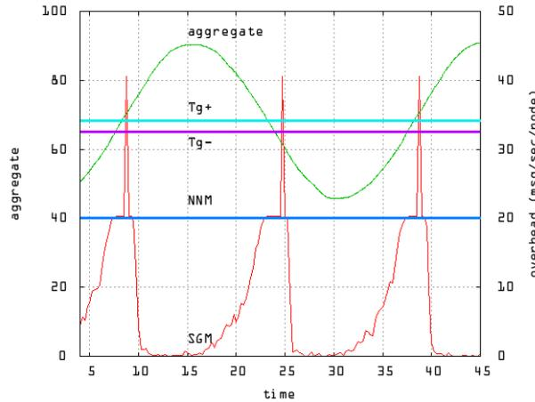
Figure 4-6: The protocol overhead over time for the SGM and NNM protocols
