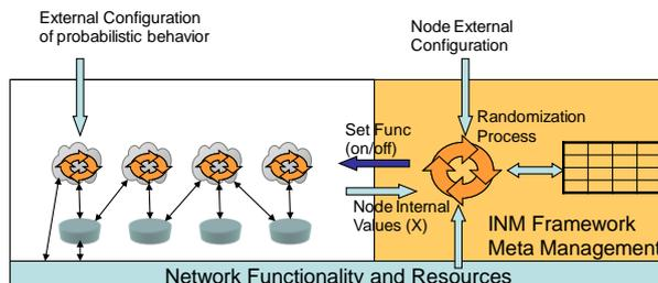
Figure 5-16: Basic probabilistic management framework (node view)
