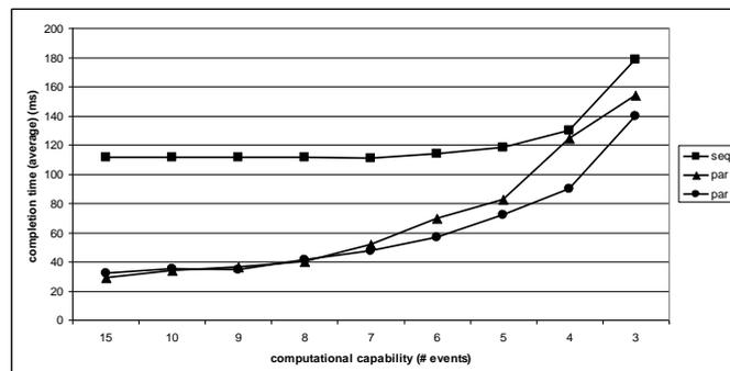
Figure 5-15: Completion time in relation to computational capability, homogeneous scenario
