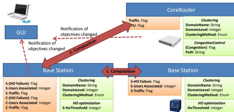
Figure 7-5: Composition steps between distributed capabilities.
