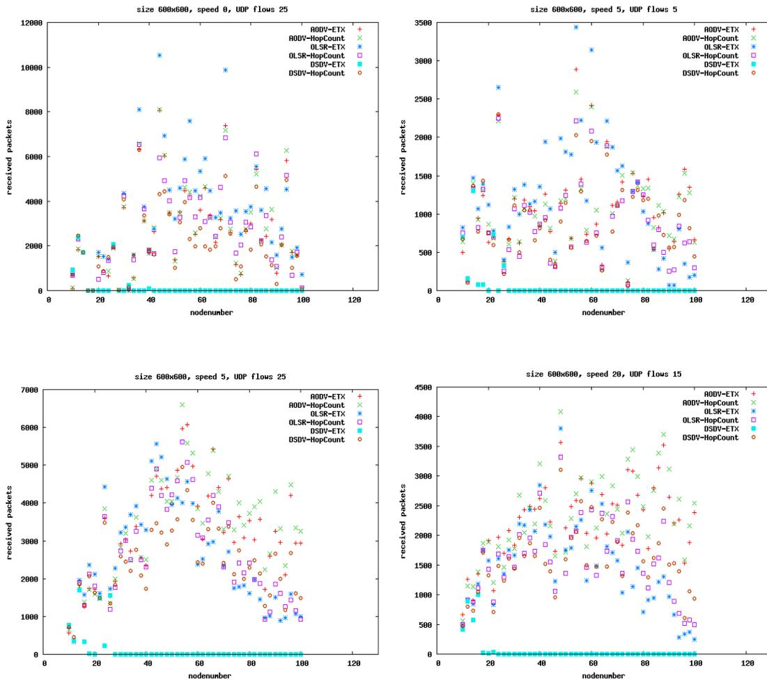
Figure D-1: Performance of AODV, OLSR, DSDV with combinations of Less Hop Count and ETX on a 600x600m square
