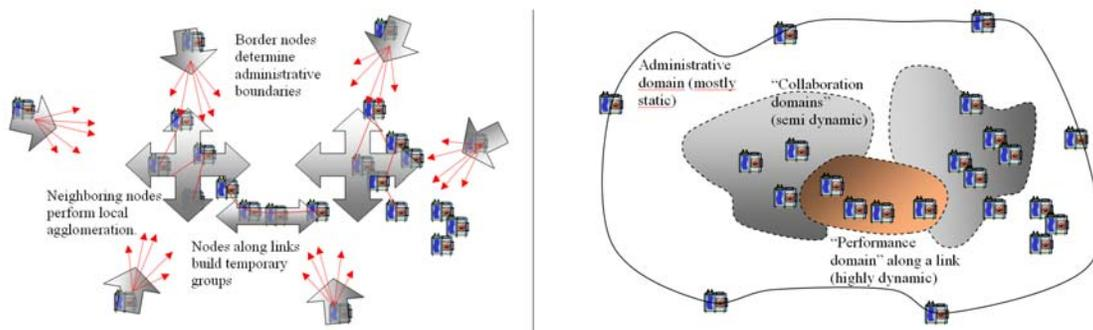
**Figure 5-7: Outside-in and inside-out methods of initiating and forming domains (left: preparation signalling; right: established domains)**
