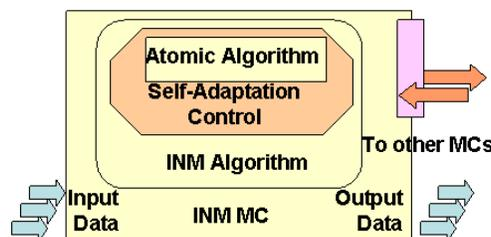
Figure 7-2: Atomic INM algorithm embedded within self-adaptation logic
