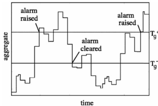
Figure 6-2: Desired threshold crossing detection functionality
