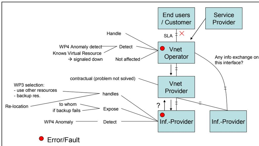
Figure 9-10: Fault Management in Vnet
