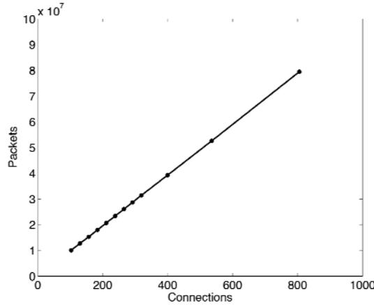
**Figure 6-8: Scalability tests for different sizes of scale-free networks.**
