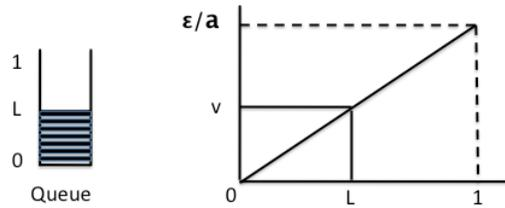
Figure C-2: Mapping of Queue Filling level to Frequency
