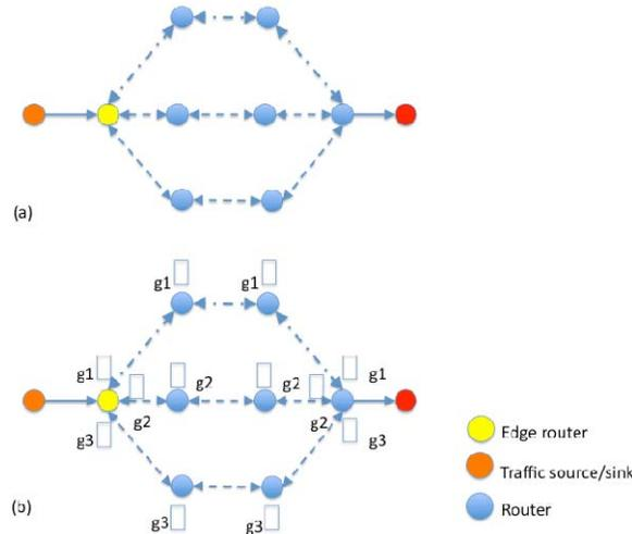
Figure C-3: Multipath-Routing Example and corresponding Oscillator Groups
