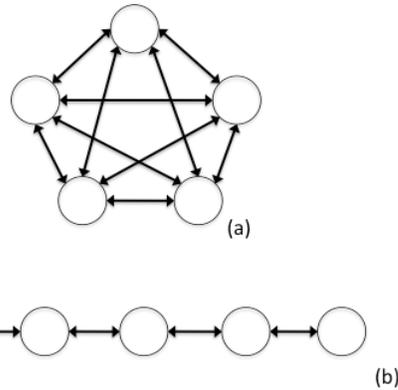
**Figure C-5: Oscillator Coupling**
