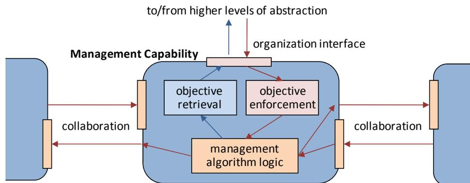
Figure 5-4: Management capabilities: structure and interaction
