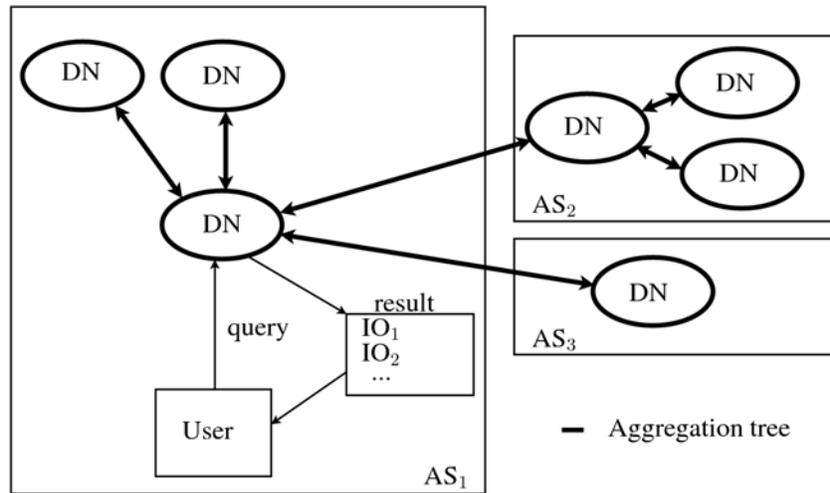
Figure 9-4: Example of metadata-directed search using tree-based aggregation.
