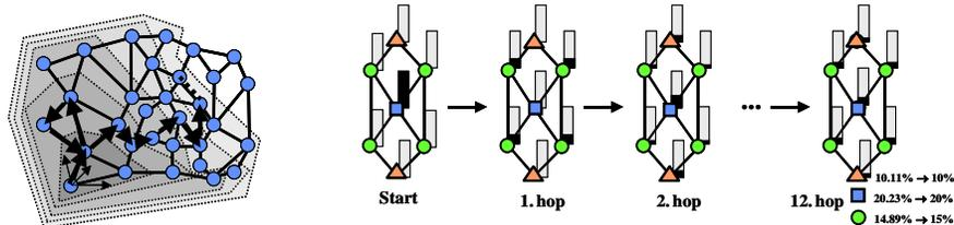
**Figure 6-7: Flooding (gray surfaces indicating distances) versus random walks (arrows)**
