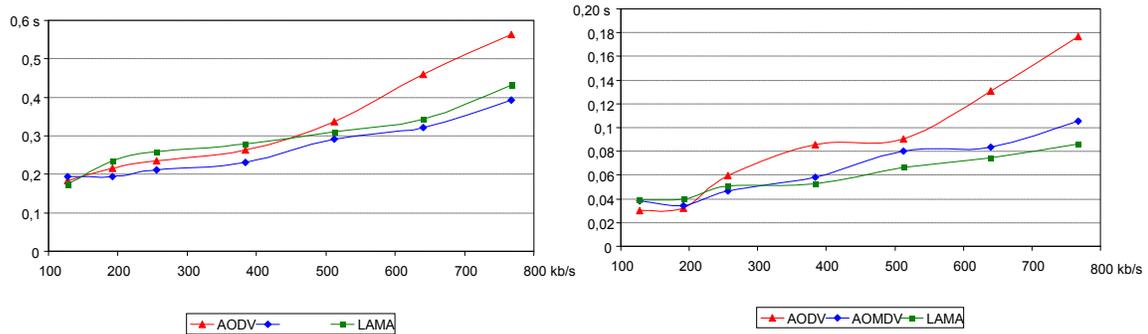
Figure 9-12 The end-to-end path delay (a) and delay jitter (b) as function of path load.
