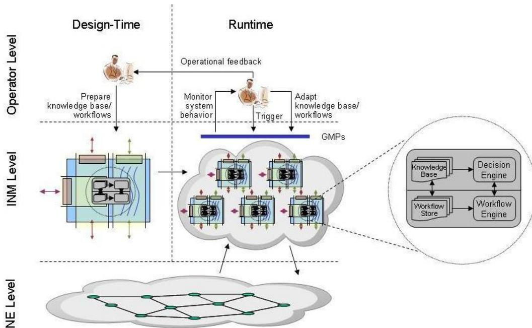
**Figure 5-9: Control of INM processes/ flows by knowledge-supported workflows**
