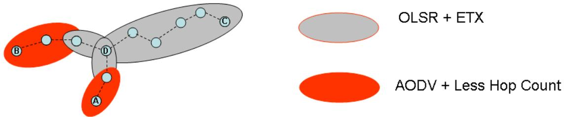
Figure 9-15: Exemplarily routing via A-HRP
