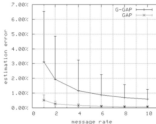
Figure 6-1: Estimation error vs. protocol overhead, from [Wuh09a]
