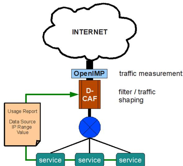
Figure 6-12: Using Valuation for Mitigating Network Overload
