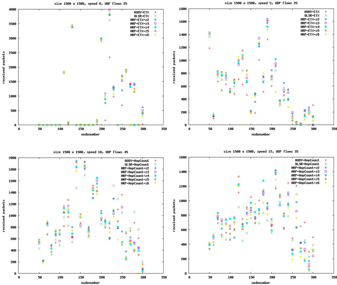
Figure D-4: Performance of AODV, OLSR and HRP with Less Hop Count on a 1500x1500m square
