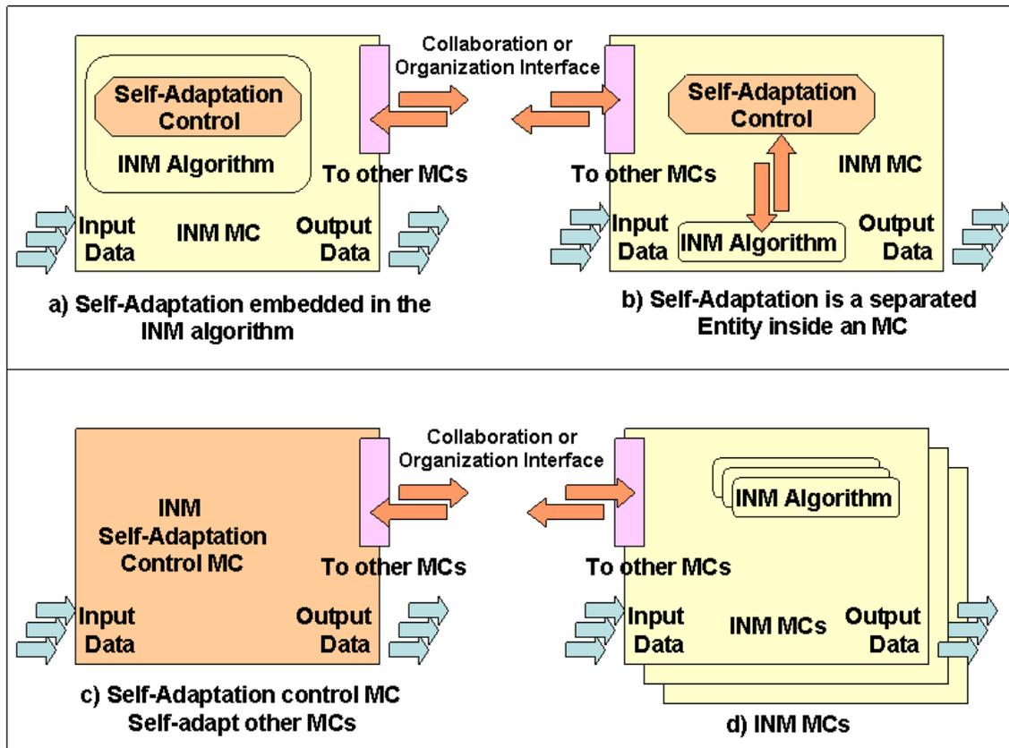
Figure 7-1: The design space of self-adaptation functionality within MCs
