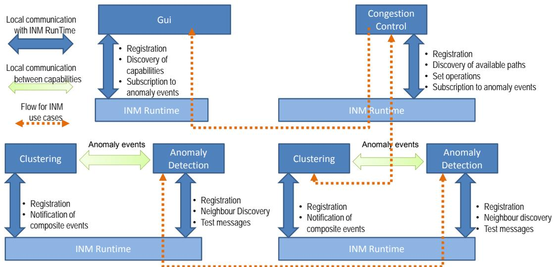
Figure 8-2: Composition of capabilities and their mapping to the prototype.
