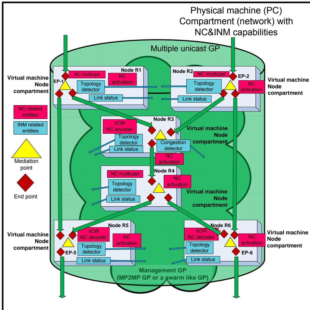
**Figure 9-13: Integration of the NC mechanism into the GP architecture**
