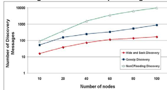
Figure 6-5: Comparison between H&S, DFS-Gossip and Non-controlled flooding approaches
