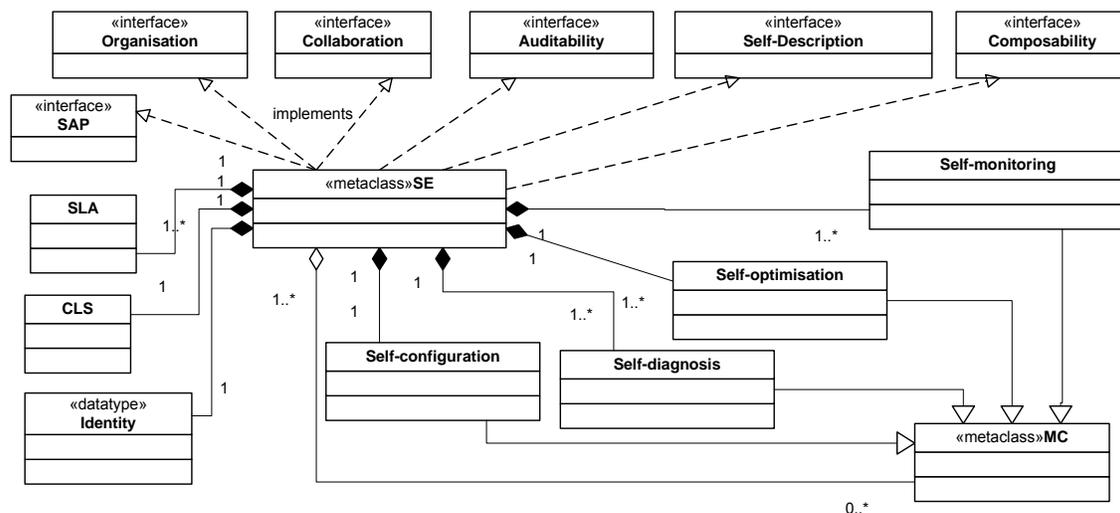
Figure 5-6: Structure of a self-managing entity.
