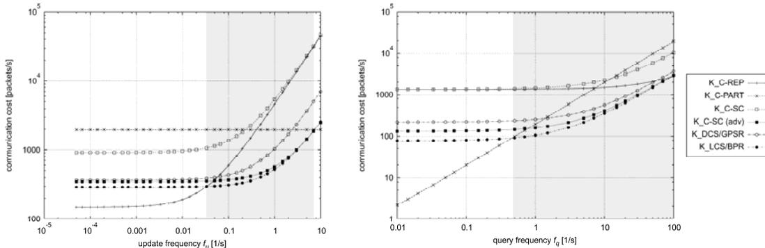
**Figure 9-3: Communication cost of data-centric storage approaches as a function of update frequency (left) and query frequency (right).**
