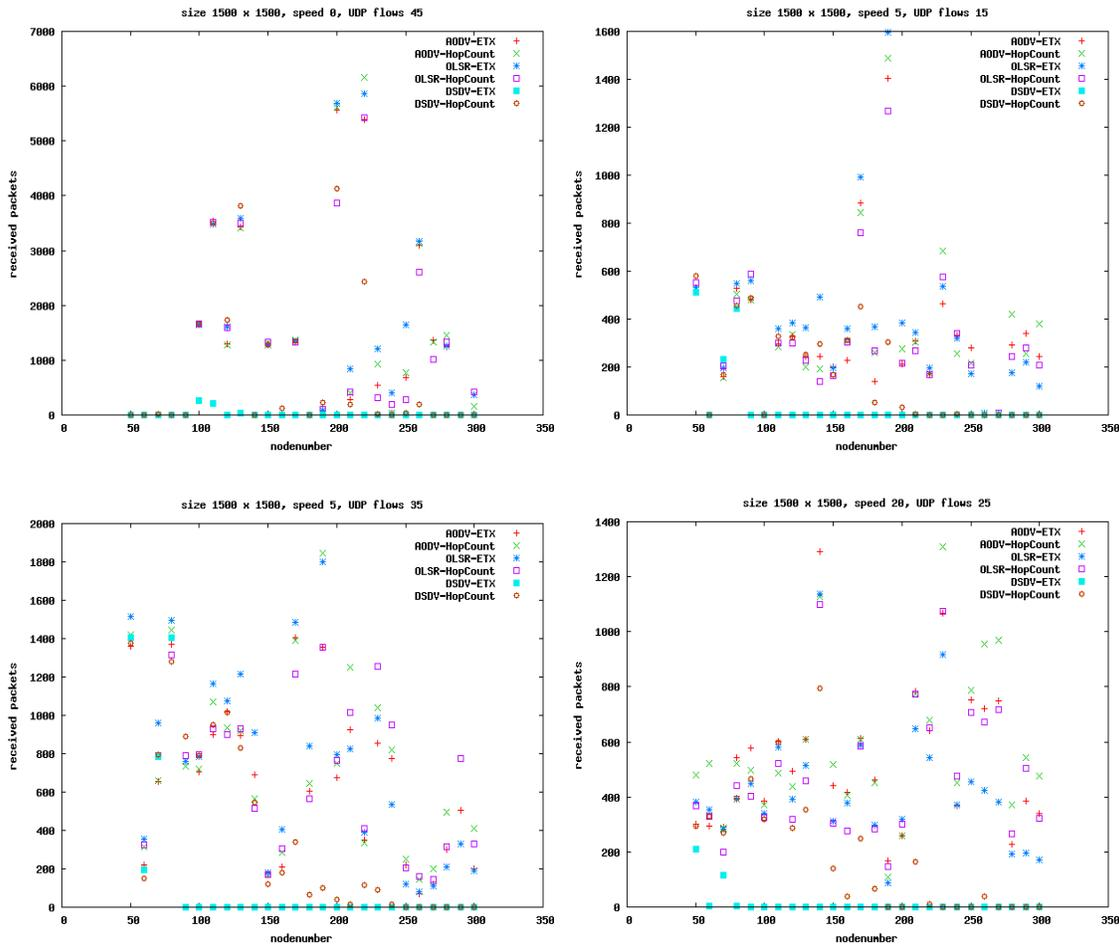
Figure D-2: Performance of AODV, OLSR, DSDV with combinations of HopCount and ETX on a 1500x1500m square
