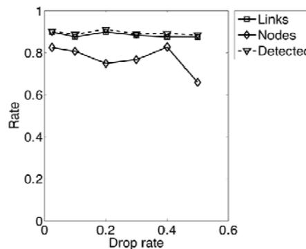
**Figure 6-10: Performance of detection and localisation of communication anomalies on links and nodes.** **Figure 6-11: Performance of detection and localization of probe response delay variations on links and nodes.**
