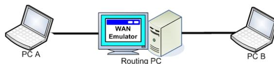
Figure 1. Testbed architecture
