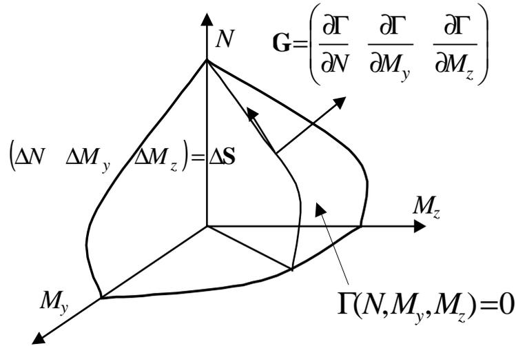
Figure 3. Yield surface of cross section
