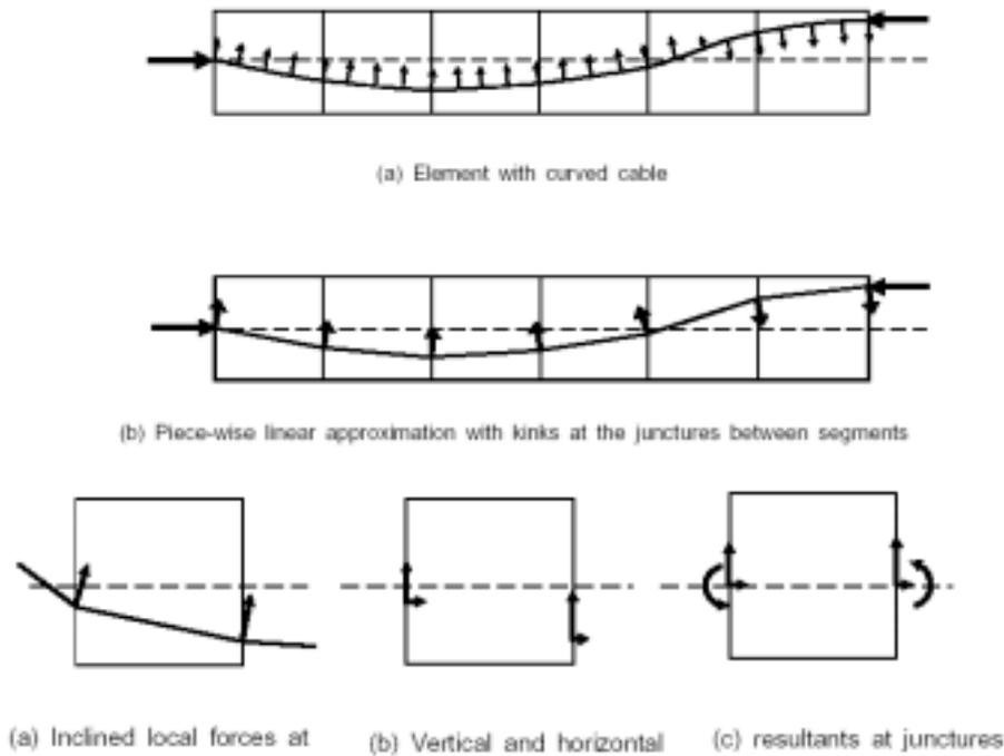
Figure 9. Typical segmented element
