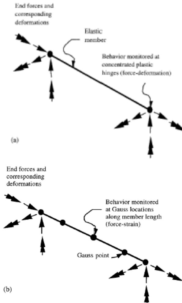
Figure 2. Beam column elements (a) Concentrated plasticity approach (b) Distributed plasticity approach
