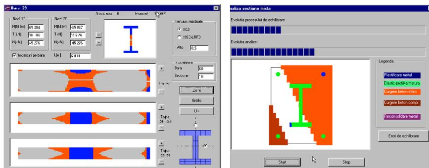
*Plot showing spread of plasticity through cross-section and along the beam column element.*
