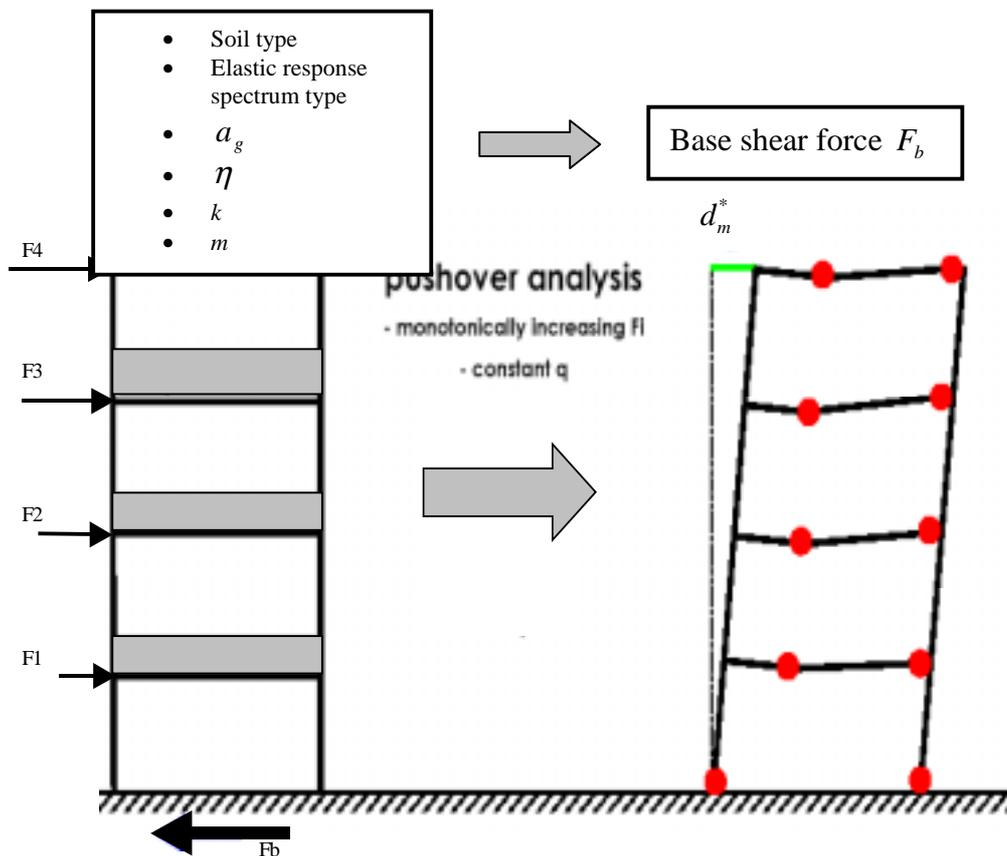
2. Idealize the pushover curve as a bilinear elasto-perfectly plastic force-displacement relationship. The yield force  $F_y^*$  is equal to the base shear force at the formation of the plastic mechanism. The initial stiffness of the idealized system is determined in such way that the areas under the actual and the idealized force-deformation curves are equal.
