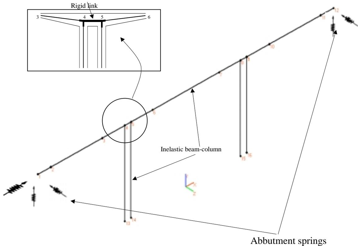
Figure 8 Structural model of the bridge
