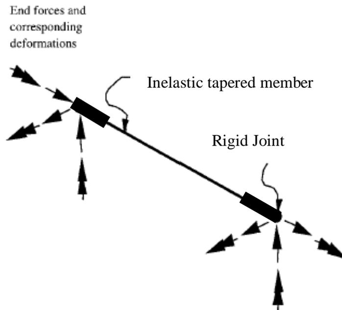
Figure 1. Typical component model
